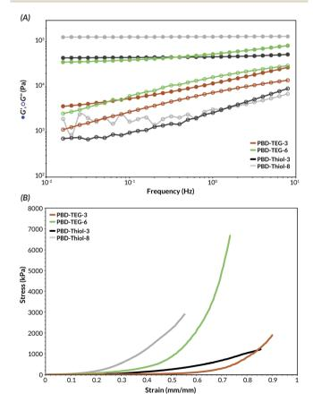
Fig. 2 (A) Frequency sweep of PBD-Thiol-X and PBD-TEG-X crosslinked specimens. (B) Compression analysis of representative PBD-TEG-X samples compared to PBD-Thiol-X.
