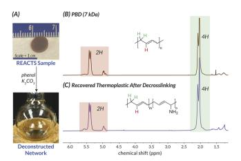
Fig. 3 (A) sample images of REACTS sample PBD-DEG-3 before and after decrosslinking.  $^1$ H NMR spectra of (B) PBD prior to REACTS crosslinking and (C) following network deconstruction of REACTS sample PBD-DEG-3. Scale bar = 1 cm.
