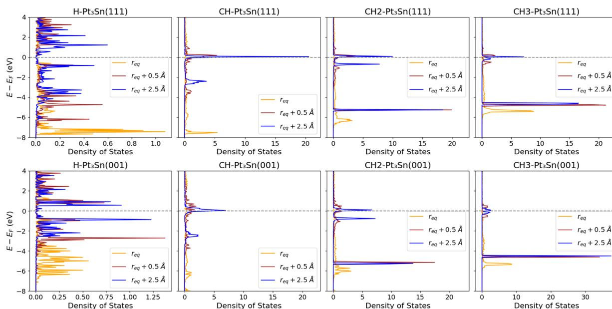
Fig. 8 Comparison of the projected adsorbate density of states on the topological surfaces of Pt<sub>3</sub>Sn at different surface-adsorbate distances.
