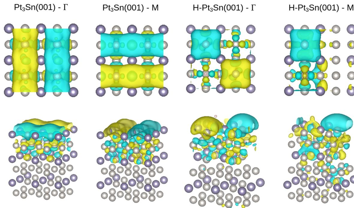
Fig. 5 Real space representation of the pristine and hydrogen adsorbed  $\text{Pt}_3\text{Sn}(001)$  ( $2 \times 2$ ) supercell surface real-valued wavefunction at high symmetry points  $\Gamma$  and  $M$ .
