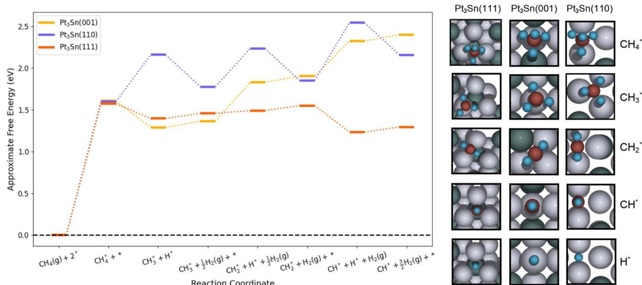
Fig. 7 Reaction profile of the dehydrogenation of methane on Pt<sub>3</sub>Sn(111), Pt<sub>3</sub>Sn(001), and Pt<sub>3</sub>Sn(110) at 1 barr and 900 K. Visualizations of the global minimum structures are given on the right hand side. Asterisks above adsorbates indicate a bound species, asterisks on their own denote a bare slab.
