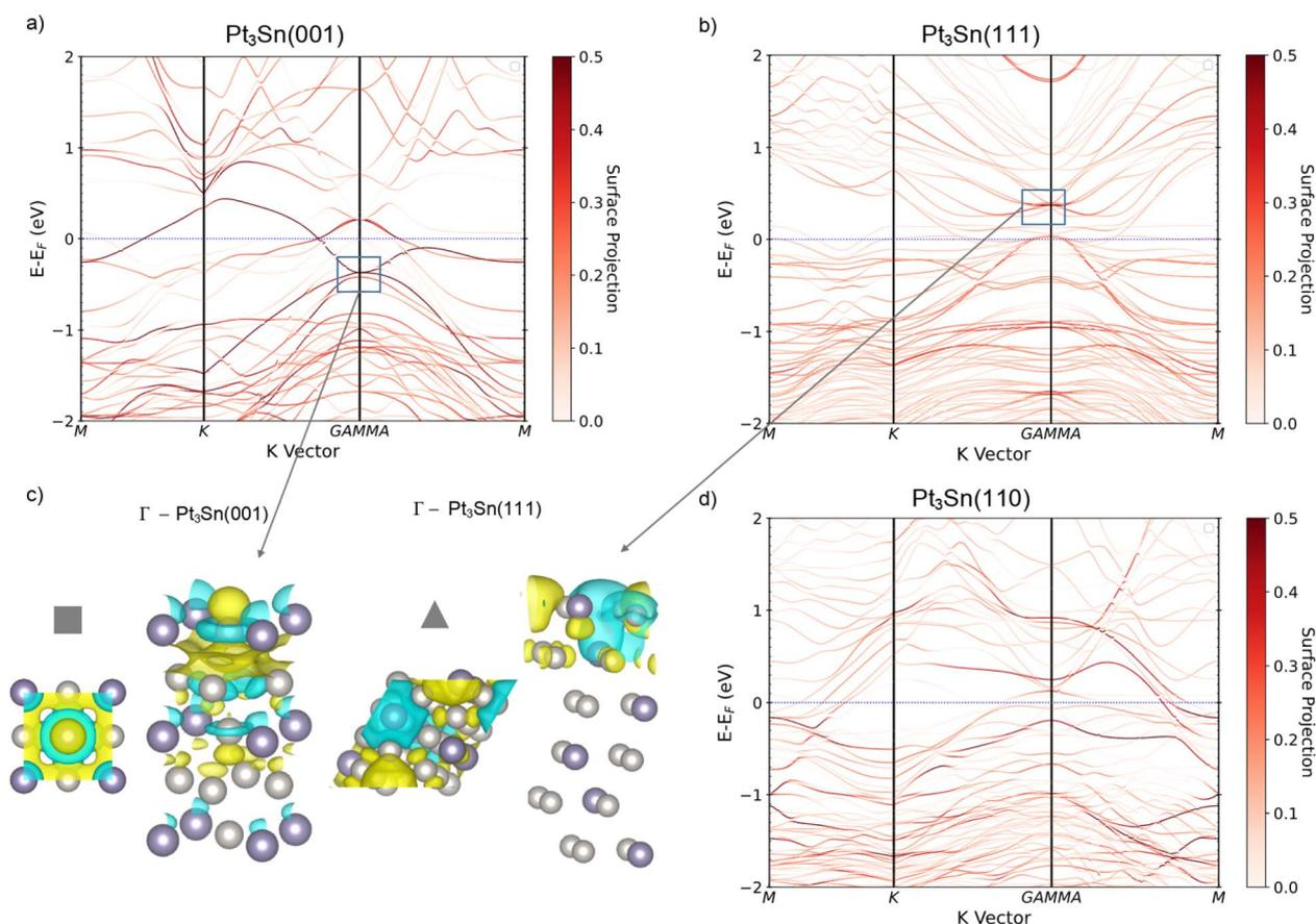
Fig. 3 Projections of the slab models for the (a) Pt<sub>3</sub>Sn(001) surface band structure, (b) Pt<sub>3</sub>Sn(111) surface band structure, (c) real space representations of the surface state wavefunctions (inset solid square) with only the topmost layers of the slab shown, (d) Pt<sub>3</sub>Sn(110) surface band structure.
