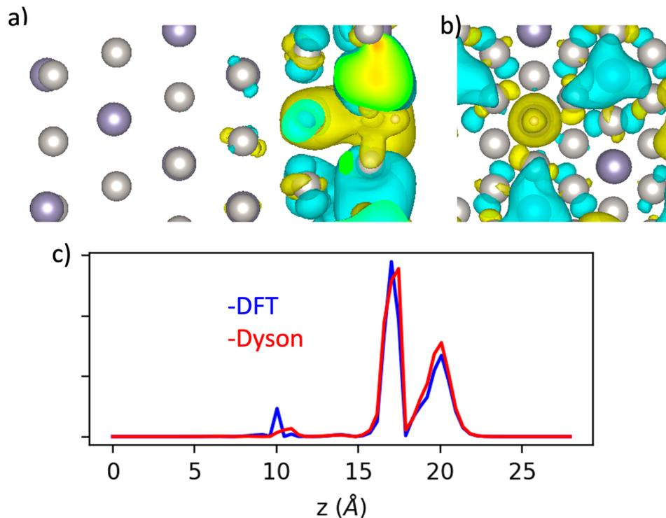
Fig. 6 The side view (a) and top view (b) of the H atom and  $\text{Pt}_3\text{Sn}$  surface atoms dominate Dyson orbital wavefunction from GW quasiparticle Hamiltonian diagonalization. (c) The  $z$  direction line profile of the charge density of the hybrid state. Blue: DFT orbital; red: Dyson orbital.
