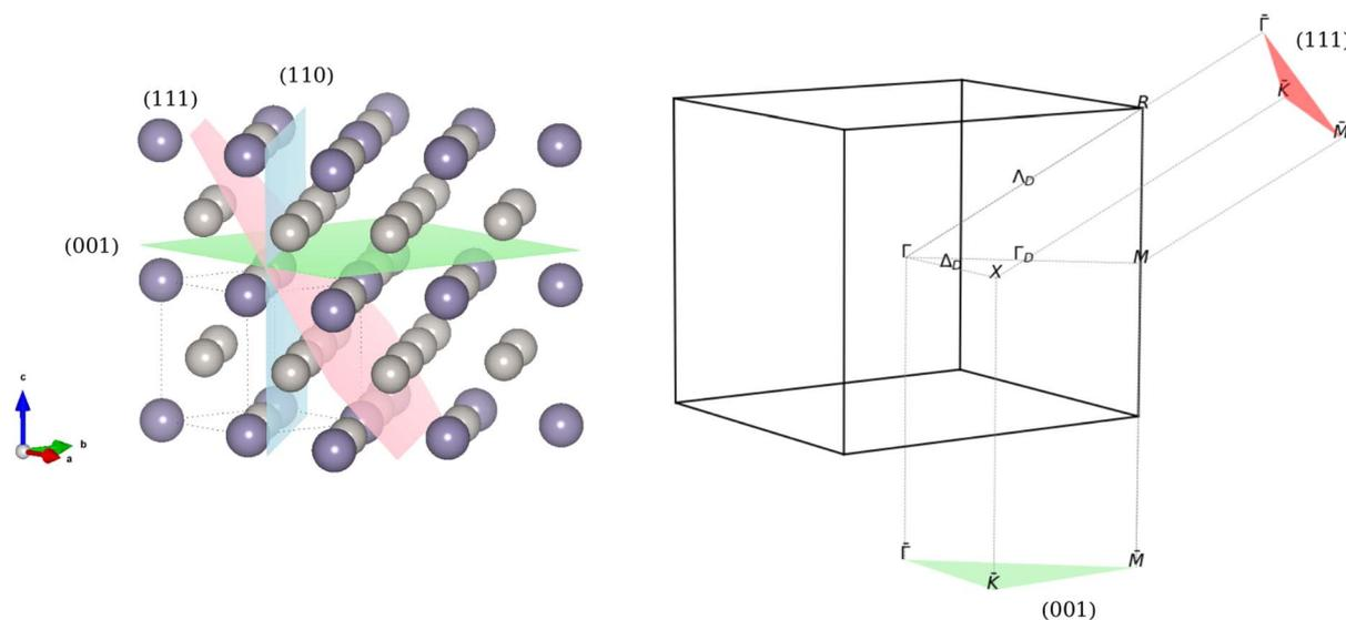
Fig. 1 (a) A Pt<sub>3</sub>Sn supercell with the (001), (111), and (110) surfaces highlighted. Sn atoms are depicted as dark blue spheres and Pt atoms are silver-grey spheres (b) depiction of the cubic reciprocal space lattice with corresponding surface projected high symmetry points. Symbols  $\Lambda_D$ ,  $\Delta_D$ , and  $T_D$  denote the location of the Dirac points on the high symmetry lines  $\Lambda$ ,  $\Delta$ , and  $T$ , respectively.
