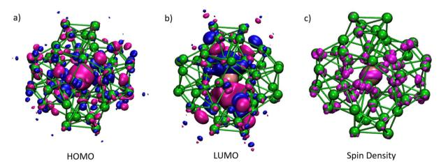
Fig. 4 (a) HOMO and (b) LUMO (magenta and blue isosurfaces) and (c) spin density (magenta isosurfaces) of the DFT-optimized  $AuCu_{56}$  NC. Only the Au (pink) and Cu (green) atoms are shown; ligands are omitted for clarity.
