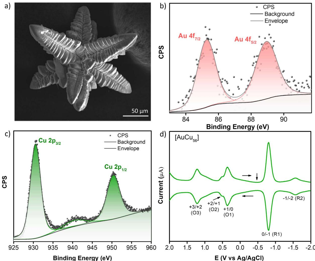
Fig. 3 (a) SEM image showing the star-shaped crystals with multiple branches. XPS spectra of the AuCu<sub>56</sub> NC showing the (b) Au 4f and (c) Cu 2p orbitals; (d) differential pulse voltammetry of [AuCu<sub>56</sub>S<sub>12</sub>(AdmS)<sub>20</sub>(O<sub>3</sub>SAdm)<sub>12</sub>] NC at a GC electrode (15 mm). DC potential ramp of 10 mV s<sup>-1</sup> and a pulse amplitude of 50 mV.
