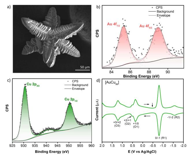
Fig. 3 (a) SEM image showing the star-shaped crystals with multiple branches. XPS spectra of the AuCu<sub>56</sub> NC showing the (b) Au 4f and (c) Cu 2p orbitals; (d) differential pulse voltammetry of  $[AuCu_{56}S_{12}(AdmS)_{20}(O_3SAdm)_{12}]$  NC at a GC electrode (15 mm). DC potential ramp of 10 mV s<sup>-1</sup> and a pulse amplitude of 50 mV.
