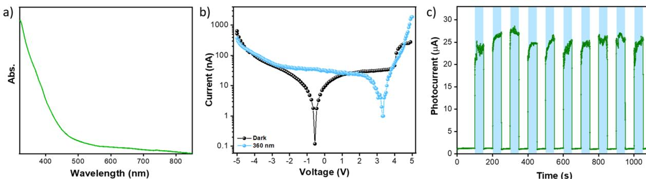
Fig. 5 (a) UV-vis absorption spectrum of the  $\text{AuCu}_{56}$  crystals dispersed in DCM. (b)  $I$ – $V$  characteristics of the device in the dark and 360 nm of laser illumination. (c) Photoresponse of the device under 360 nm laser irradiation, with the arrows indicating the response and recovery time of the device.
