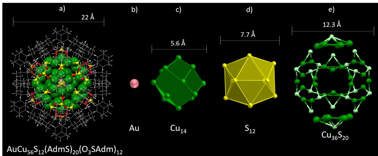
Fig. 1 Overview of the atomic structure of the  $\text{AuCu}_{56}$  NC. (a) Total structure of the  $\text{AuCu}_{56}$  NC. (b) The innermost Au atom present inside the (c)  $\text{Cu}_{14}$  cuboctahedron which is then connected to (d) a layer of  $12 \text{ S}^{2-}$  arranged in the shape of an icosahedron. (e) The atomic structure of the  $\text{Cu}_{36}\text{S}_{20}$  outermost layer. Color code: pink, Au; green, Cu; yellow and light green, S; red, O; gray, C; white, H.
