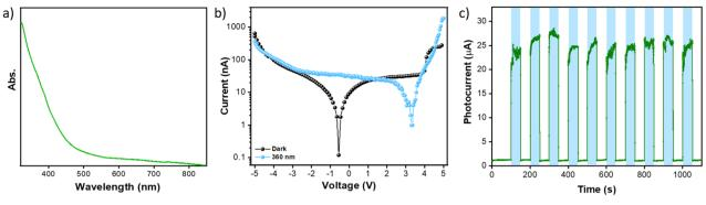
Fig. 5 (a) UV-vis absorption spectrum of the  $AuCu_{56}$  crystals dispersed in DCM. (b) I-V characteristics of the device in the dark and 360 nm of laser illumination. (c) Photoresponse of the device under 360 nm laser irradiation, with the arrows indicating the response and recovery time of the device
