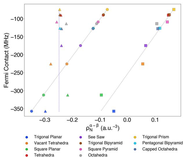
Fig. 10 Correlation between Fermi contact contribution and total nuclear spin density for  $[V(NH_3)_x]^{4+}$  (where  $x = 3-7$ ) compounds. Squares, triangles, and circles represent the valence shell, core–shell and total contributions, respectively. Numerical details can be found in Table S17.†
