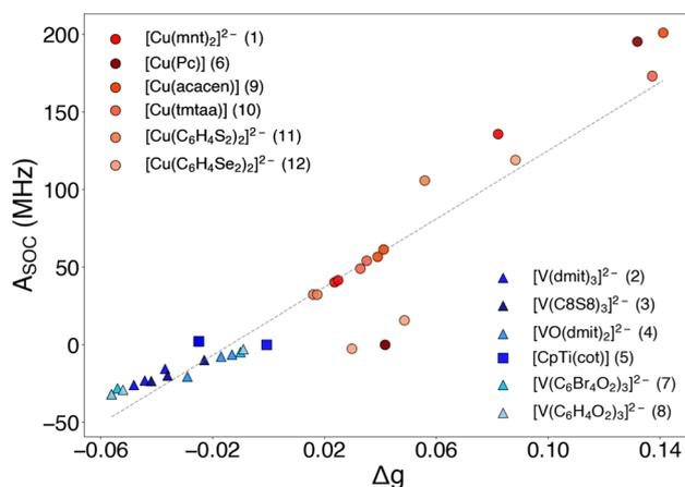
Fig. 8 Computed  $\Delta g_{\mu\nu}$  against total  $A_{\mu\nu}^{\text{SOC}}$  (where  $\mu = \nu$ ) for compounds 1–12. All calculations were performed using a fully uncontracted ANO-DK3 basis set and B3LYP employing a ZORA relativistic treatment.
