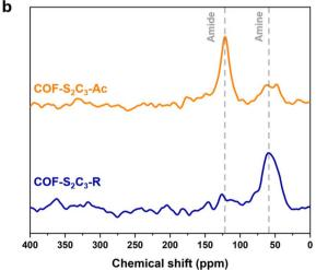
Fig. 4 (a)  $^{13}$ C CP-MAS ssNMR spectra and (b)  $^{15}$ N CP-MAS ssNMR spectra for COF-S $_2$ C $_3$ -R (blue) and COF-S $_2$ C $_3$ -Ac (orange).
