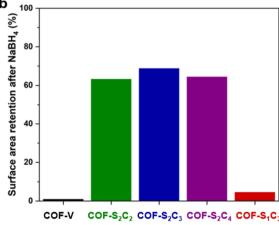
Fig. 3 (a)  $N_2$  sorption isotherms at 77 K (filled circles show adsorption and open circles show desorption) for the reported materials after treatment with NaBH<sub>4</sub> and (b) retention of BET surface area (%) for after NaBH<sub>4</sub> treatment.
