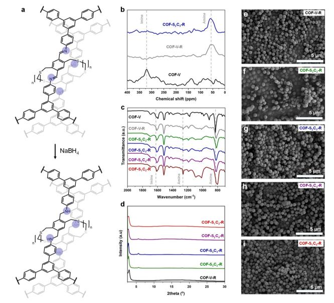
Fig. 2 (a) Chemical structure (n = 2, 3, or 4) for the crosslinked materials before and after imine reduction. (b) <sup>15</sup>N CP-MAS ssNMR spectra, (c) FTIR spectra, (d) PXRD patterns, and (e-i) SEM images for COF-V-R, COF-S<sub>2</sub>C<sub>2</sub>-R, COF-S<sub>2</sub>C<sub>3</sub>-R, COF-S<sub>2</sub>C<sub>4</sub>-R, and COF-S<sub>1</sub>C<sub>3</sub>-R.
