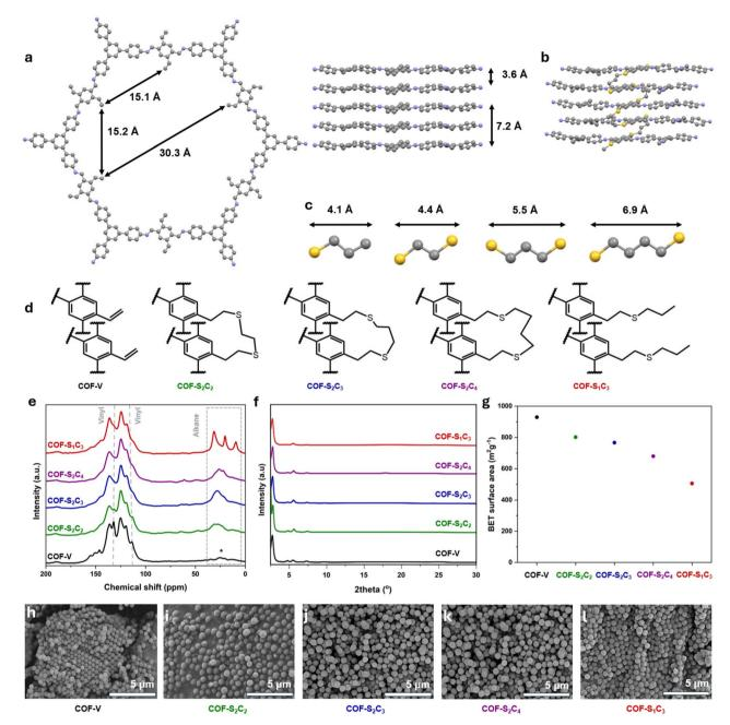
Fig. 1 (a) Simulated structure of COF-V. (b) Simulated structure of COF-S<sub>2</sub>C<sub>3</sub>. (c) Simulated structure of dithiol crosslinkers. (d) Chemical structures of reported materials. (e)  $^{13}$ C CP-MAS ssNMR spectra, (f) PXRD patterns, (g) BET surface areas, and (h–l) SEM images for the reported materials.
