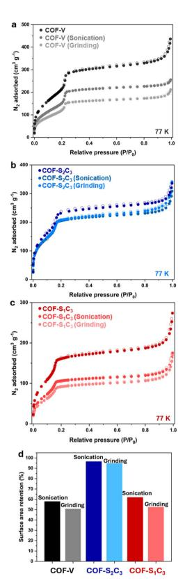
Fig. 5  $N_2$  sorption isotherms of (a) COF-V, (b) COF-S<sub>2</sub>C<sub>3</sub>, and (c) COF-S<sub>1</sub>C<sub>3</sub> before and after mechanical treatment. Filled circles show adsorption and open circles show desorption. (d) Retention of BET surface area (%) after mechanical stability tests for COF-V, COF-S<sub>1</sub>C<sub>3</sub>, and COF-S<sub>2</sub>C<sub>3</sub>.
