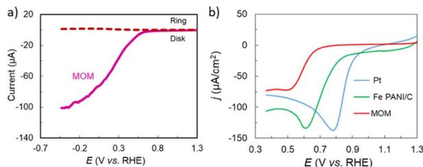
Fig. 5 (a) Rotating ring disk electrochemistry (RRDE) plots for the ORR of MOM **1** at pH = 13 and 300 rpm. Solid and dashed lines are the disk and ring currents, respectively. (b) Electrocatalytic ORR activity of MOM, Pt, and Fe PANI/C in air-saturated 0.1 M KOH. Experimental conditions: Pt wire and Ag/AgCl were used as the counter and reference electrodes, respectively.
