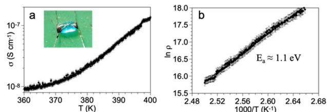
Fig. 4 (a) Thermal variation of the electrical conductivity of MOM **1**. Inset shows a picture of one of the single crystals used for the measurements. (b) Arrhenius plot of MOM **1** in the temperature range 400–375 K.
