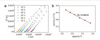
Fig. 3 (a) Nyquist plots of a pellet of MOM  $\bf 1$  at 98% RH and different temperatures in the range 25–75 °C. (b) Arrhenius plot of the proton conductivity of  $\bf 1$  at 98% RH in the temperature range 25–75 °C.
