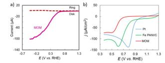
Fig. 5 (a) Rotating ring disk electrochemistry (RRDE) plots for the ORR of MOM  ${\bf 1}$  at pH = 13 and 300 rpm. Solid and dashed lines are the disk and ring currents, respectively. (b) Electrocatalytic ORR activity of MOM, Pt, and Fe PANI/C in air-saturated 0.1 M KOH. Experimental conditions: Pt wire and Ag/AgCl were used as the counter and reference electrodes, respectively.
