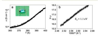
Fig. 4 (a) Thermal variation of the electrical conductivity of MOM 1. Inset shows a picture of one of the single crystals used for the measurements. (b) Arrhenius plot of MOM 1 in the temperature range 400-375 K.
