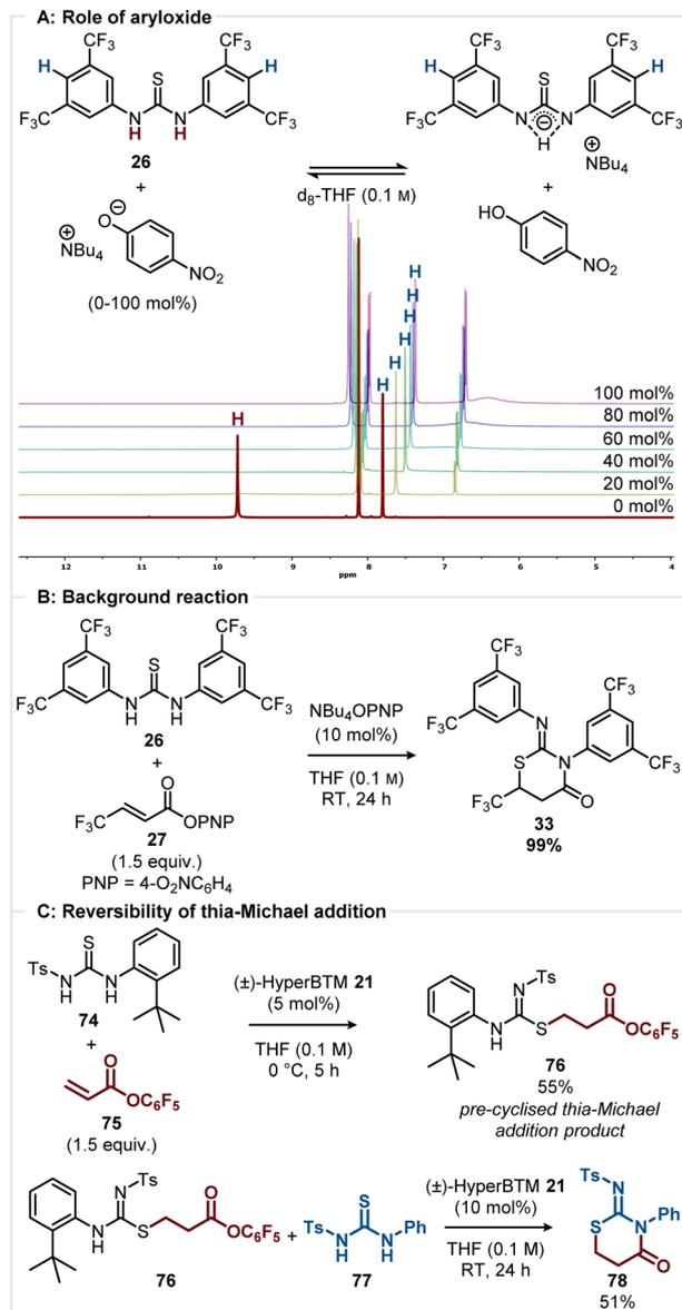
Scheme 5 (A) Determining role of aryloxide by  $^1\text{H}$  NMR titration. (B) Aryloxide catalysed racemic background reaction. (C) Probing reversibility of the thia-Michael addition by crossover experiment.
