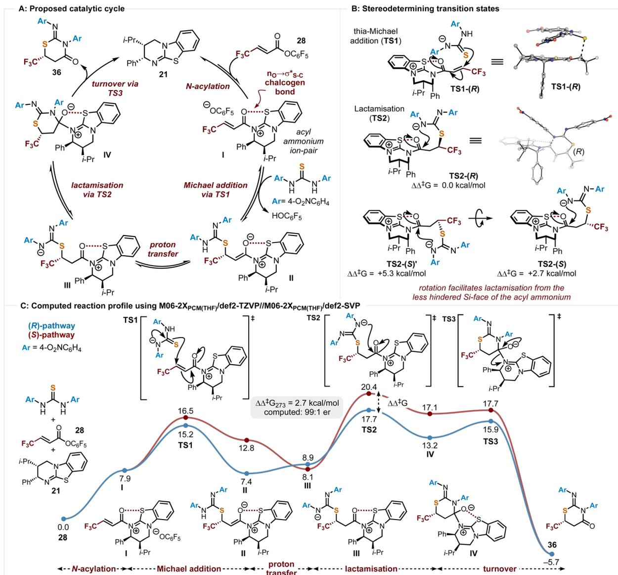
Scheme 6 (A) Proposed catalytic cycle. (B) DFT analysis of the stereodetermining transition state. (C) Computed reaction profile leading to enantiomeric products. M06-2X<sub>SMD(THF)</sub>/def2-TZVP//M06-2X<sub>SMD(THF)</sub>/def2-SVP Gibbs free energies ( $\Delta G_{273}$ ) shown in kcal mol<sup>-1</sup>.
