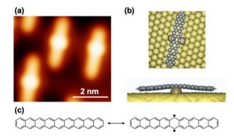
Fig. 10 (a) STM image of nonacene—Au interaction. (b) Side and top views of the corresponding DFT equilibrium geometry. (c) Closed-shell Kekulé (left) and one of the many possible non-Kekulé (right) Clar structures of nonacene. Adapted with permission from ref. 57. Copyright 2019 Springer Nature.
