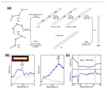
Fig. 17 (a) Synthetic strategy for pentadecacene. (b) d//dV curves for pentadecacene; two resonance peaks are identified as the HOMO and LUMO. (c) Low-bias d//dV curve (top) and its corresponding d²//dV² spectrum. Adapted with permission from ref. 72. Copyright 2025 American Chemical Society.
