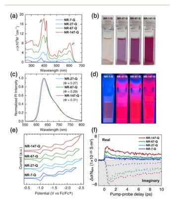
Fig. 45 (a) UV-vis absorption and (c) fluorescence spectra of molecular GNRs in CHCl<sub>3</sub>. (b) 5 mM solutions of GNRs in CHCl<sub>3</sub> under natural light and (d) UV light. (e) Cyclic voltammograms of the GNRs in n-Bu<sub>4</sub>NPF<sub>6</sub>/CH<sub>2</sub>Cl<sub>2</sub>. (f) Time-resolved THz photoconductivity ( $\Delta \sigma$ ) of different GNRs normalized to absorbed photon density following resonant excitation. Adapted with permission from ref. 184. Copyrights 2023 Cell Press.
