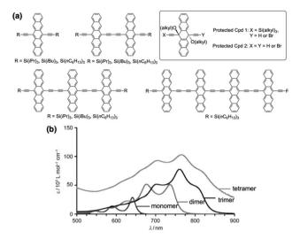
Fig. 39 (a) Pentacene oligomers employed in this study. Protected building blocks are also shown. (b) Absorption spectra of oligomers.  $R=Si(nC_6H_{13})_3$ . Adapted with permission from ref. 147. Copyright 2012 Wiley.
