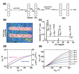
Fig. 38 (a) Synthesis of ethynylene-bridged pentacene dimers. (b) Optical microscope image of dip-coated dimer films on a Si/SiO $_2$  substrate. (c) Out-of-plane XRD patterns of dip-coated dimer films. (d) Representative transfer characteristics of the device at a fixed  $V_{\rm SD}=-60\,$  V. (e) Representative output characteristics of the device. Reproduced with permission from ref. 145. Copyright 2018 Wiley.
