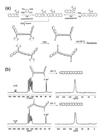
Fig. 26 (a) Synthetic route for nonacene precursors. (b) Thermal decarbonylation of precursors at 350 °C for 20 min and <sup>13</sup>C CP-MAS NMP spectra. Adapted with permission from ref. 99. Copyright 2022 Springer Nature.
