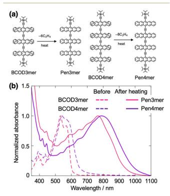
Fig. 41 (a) Thermal conversion. (b) Representative normalized absorption spectra of BCDO3mer and BCOD4mer before and after heating in diphenyl ether. Heating conditions: 300 °C, 3 minutes for BCOD3mer, and 260 °C, 5 minutes and then 280 °C, 90 seconds for BCOD4mer under a  $\rm N_2$  atmosphere. Adapted with permission from ref. 151. Copyright 2024 Wiley.
