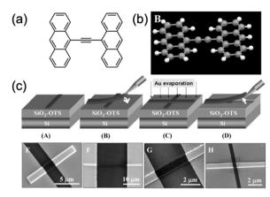
Fig. 33 (a) Chemical structure of di-anthrylene-ethynylene. (b) Single crystal X-ray structure. (c) Schematic of device fabrication by using the "organic ribbon mask" technique, and SEM images of devices with different channel lengths by using the technique. Adapted with permission from ref. 127. Copyright 2008 Wiley.
