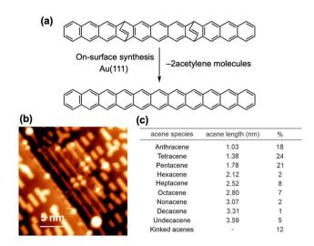
Fig. 15 (a) On-surface synthesis of undecacene from an ethenobridged precursor. (b) Overview STM topography image after annealing the sample at 220 °C. (c) Table showing the statistics of the acene species found on the substrate after annealing at 220 °C. Adapted with permission from ref. 71. Copyright 2022 Springer Nature.
