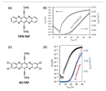
Fig. 42 (a) Molecular structure of TIPS-TAP. (b) Transfer characteristics of the device for a thin-film transistor with TIPS-TAP at a fixed  $V_{\rm SD} = -60$  V. (c) Molecular structure of 4Cl-TAP. (d) Transfer characteristics of the device for a thin-film transistor of 4Cl-TAP with the highest field effect mobility. Adapted with permission from ref. 166 for (b), and ref. 165 for (d). Copyrights 2011 Wiley for (b) and 2018 Wiley for (d).
