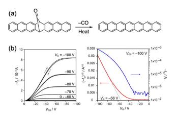
Fig. 31 (a) Heptacene generation from its monoketone precursor. (b) Output (left) and transfer characteristics (right,  $V_{\rm DS}=-100$  V) of heptacene thin films. Adapted with permission from ref. 114. Copyright 2021 Wilev.
