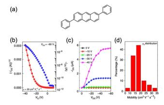
**Fig. 32** (a) Chemical structure of 2,6-diphenylanthracene. Typical (b) transfer and (c) out-put characteristics of the SCFET device based on 2,6-diphenylanthracene. (d) Mobility distribution. Reproduced with permission from ref. 119. Copyright 2015 Spring Nature.
