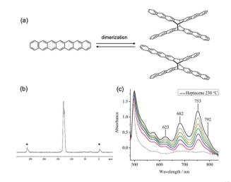
Fig. 24 (a) Heptacene and its dimerization reaction. (b) Solid state <sup>13</sup>C CP-MAS NMR spectrum. The sample was stored at room temperature in an ambient atmosphere for 1 month, and then heated at 300 °C for 12 min. (c) Absorption spectra of heptacene obtained by heating a solution of diheptacene in 1-methylnaphthalene. Adapted with permission from ref. 97. Copyright 2017 American Chemical Society.
