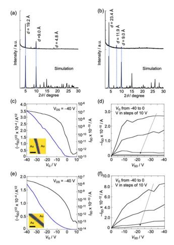
Fig. 36 (a and b) Experimental out-of-plane XRD and simulated powder XRD patterns of (a) 3mer and (b) 4mer single crystals on a Si/ SiO<sub>2</sub>/OTS substrate. (c and e) Transfer characteristics of the device for (c) 3mer and (e) 4mer at a fixed source/drain voltage,  $V_{SD} = -40 \text{ V}$ . (d and f) Output characteristics of the device for (d) 3mer and (f) 4mer. Reproduced with permission from ref. 136. Copyright 2021 Wiley.
