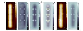
Fig. 18 (a) (Left to right) STM, constant-current nc-AFM, and constant-height nc-AFM of the 6Au-pentadecacene complex. (b) Constant-height nc-AFM image with the chemical structure. (c) STM and constant-height nc-AFM image of the 5Au-pentadecacene complex, which was obtained by removing a single Au atom from the 6Au-pentadecacene complex. Reproduced with permission from ref. 72. Copyright 2025 American Chemical Society.
