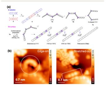
Fig. 16 (a) Synthetic strategy for tridecacene. (b) Magnified constantcurrent STM image of edge-on and stretched-out conformations of a tridecacene precursor. Reproduced with permission from ref. 73. Copyright 2024 American Chemical Society.
