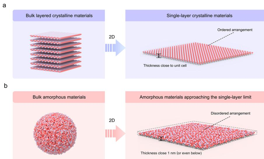
**Fig. 1** Thinning of bulk materials to the single-layer limit. (a) Thinning of bulk layered materials to obtain a stable crystalline single-layer, with a unit-cell thickness. (b) Thinning of bulk amorphous materials approaching the single-layer limit. In the atomically thin amorphous system, the intrinsically disordered structure will be well preserved (stochastic atomic packing, exemplified by Zachariasen's continuous random network (Z-CRN)).
