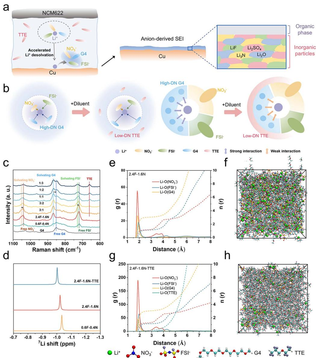
**Fig. 1** (a) A LHCE with dual salts based on a DN modulation rule and the promoted stable SEI. (b) Schematic illustration of the strong solvation effect of G4 and the shielding effect of TTE. (c) Raman spectra. (d)  $^7\text{Li}$  NMR spectra. Radial distribution functions and corresponding coordination numbers of (e) 2.4F-1.6N and (g) 2.4F-1.6N-TTE electrolytes. (f) and (h) Corresponding MD-simulated snapshots of (e) and (g), respectively.
