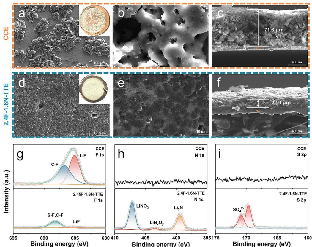
Fig. 3 Top views of Li deposited in (a) and (b) CCE and (d) and (e) 2.4F-1.6N-TTE electrolytes. The inset shows an optical image of Li deposited on copper foil. The cross-sectional SEM images on the deposited Li metal in electrolytes of (c) CCE and (f) 2.4F-1.6N-TTE. XPS spectra of (g) F<sub>1s</sub>, (h) N<sub>1s</sub> and (i) S<sub>2p</sub> on the Li-metal anode at 0.5 mA cm<sup>-2</sup>, 0.5 mA h cm<sup>-2</sup> after 10 cycles.
