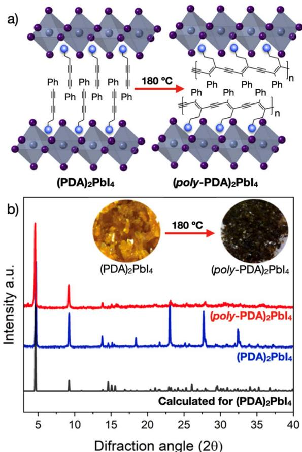
Fig. 2 (a) Schematic representation of the polymerization process of  $(\text{PDA})_2\text{PbI}_4$  to form  $(\text{poly-PDA})_2\text{PbI}_4$ . (b) Powder X-ray diffraction of  $(\text{PDA})_2\text{PbI}_4$  (blue line),  $(\text{poly-PDA})_2\text{PbI}_4$  (red line) and the calculated PXRD pattern of  $(\text{PDA})_2\text{PbI}_4$  crystal structure. Inset: photographs of  $(\text{poly-PDA})_2\text{PbI}_4$  and  $(\text{PDA})_2\text{PbI}_4$ .
