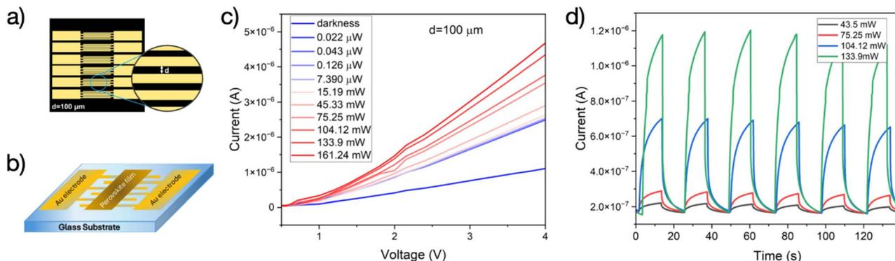
Fig. 3 (a) Interdigitated electrode architecture and (b) and schematic device architecture (c). Current–voltage ( $I$ – $V$ ) characteristics of the photodetector at varying bias voltages and laser optical powers (at 980 nm) for an interelectrode spacing of 100  $\mu\text{m}$ . (d) Temporal photoresponse of the photodetector under a 4 V bias voltage at different optical power levels (also at 980 nm).
