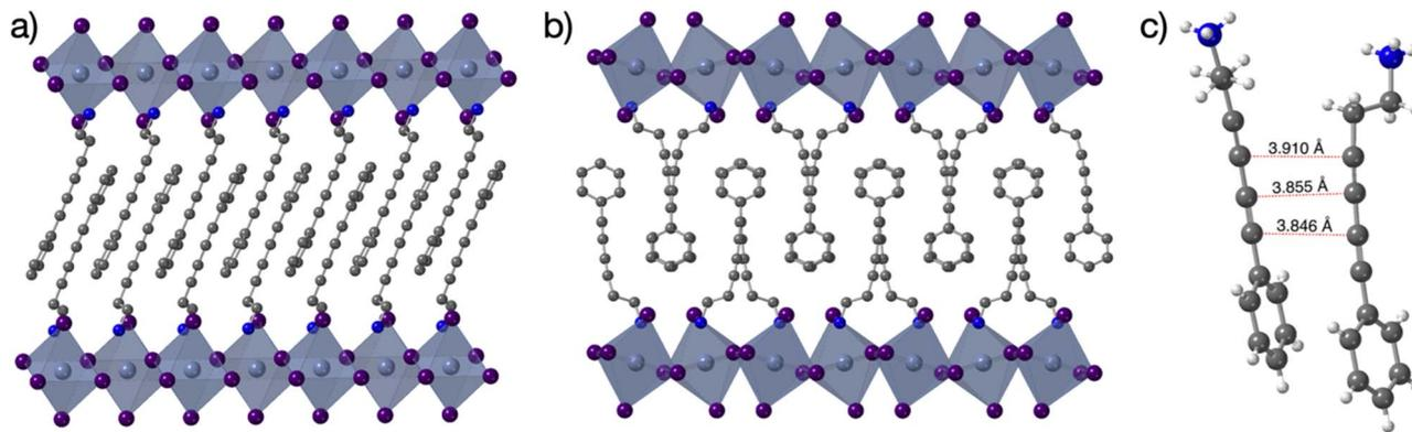
Fig. 1 (a) and (b) Crystal structure of  $(\text{PDA})_2\text{PbI}_4$  seen from b and c, respectively (a and b). Hydrogen-bonds were omitted for clarity. Purple: iodine, light blue: lead, dark blue: nitrogen, grey: carbon. (c) Selected  $\text{Csp}\cdots\text{Csp}$  distances found within the structure of  $(\text{PDA})_2\text{PbI}_4$ , dark blue: nitrogen, grey: carbon, white: hydrogen.
