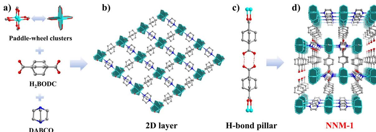
Fig. 1 The assembly and structure of **NNM-1**: (a) three starting components for the assembly of **NNM-1**; (b) two-dimensional (4, 4)-squared layer; (c) hydrogen-bonded pillar (a pair of HBODC<sup>-</sup>); (d) double-interpenetrated structure of **NNM-1**. Color codes: Cu, sky blue; C, gray; H, white; O, red; and N, blue.
