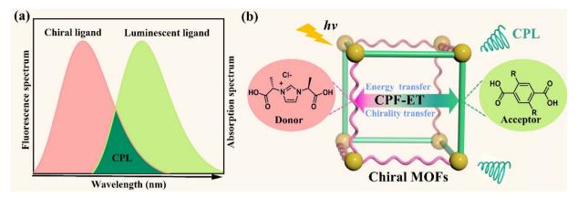
Scheme 1 (a) Schematic illustration of the CPL mechanism within CPF-ET. (b) Our design strategy of CPL-active CMOFs via CPF-ET.
