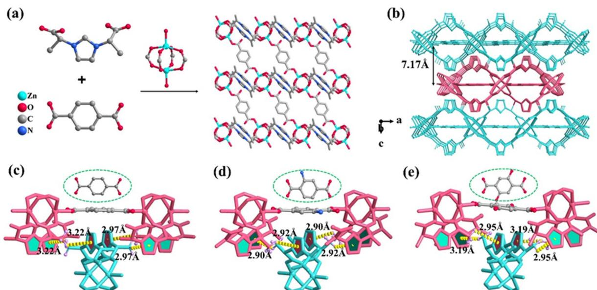
Fig. 1 (a) Diagrams illustrating the secondary building units and layer structures of L-1. (b) 3D stacking diagrams along the *b*-axis of L-1. (c)–(e) The C–H– $\pi$  interaction between adjacent layers of L-1, L-2, and L-3.
