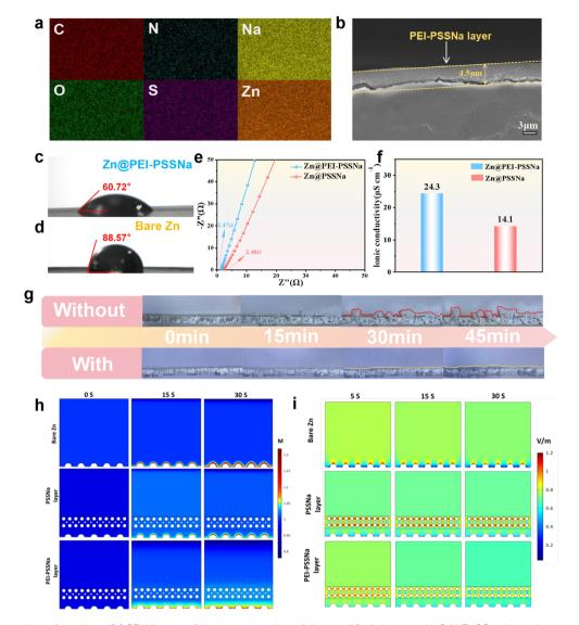
Fig. 4 (a) EDS mapping of coatings. (b) SEM image of the cross-section of the modified zinc anode. 2 M ZnSO<sub>4</sub> electrolyte contact angle on (c) Zn@PEI-PSSNa and (d) bare Zn. (e) Nyquist plots of samples at room temperature. (f) Ionic conductivity of the sample. (g) In situ optical image of the sample at a current density of 10 mA cm $^{-2}$ . (h) Simulation of the Zn concentration field at different electrodes. (i) Simulation of the electric field on different electrodes
