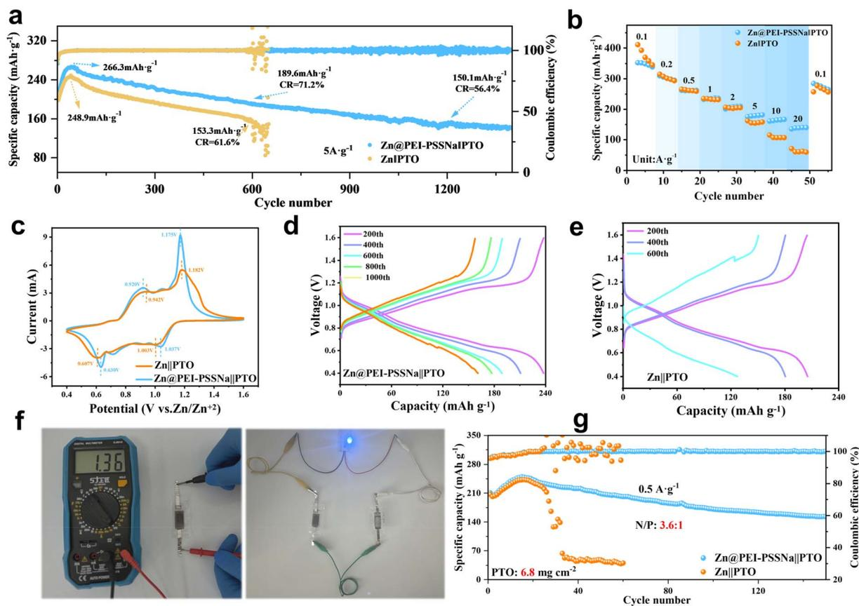
Fig. 5 (a) Comparative cycling performance of full batteries at a current density of 5 A g<sup>-1</sup>. (b) Multiplier performance test for full batteries. (c) CV curves for the full batteries at 1 mV s<sup>-1</sup> sweep speed. Charge–discharge curves of the full batteries using (d) Zn@PEI-PSSNa and (e) bare Zn anode. (f) Test photo of the small pouch-cell and (g) cycling performance of the pouch cell at a high mass loading of the cathode material.
