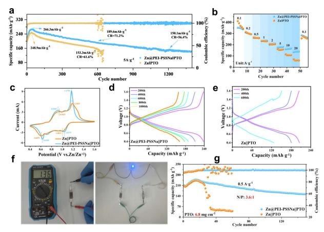
Fig. 5 (a) Comparative cycling performance of full batteries at a current density of  $5 \text{ A g}^{-1}$ . (b) Multiplier performance test for full batteries. (c) CV curves for the full batteries at 1 mV s<sup>-1</sup> sweep speed. Charge–discharge curves of the full batteries using (d) Zn@PEI-PSSNa and (e) bare Zn anode. (f) Test photo of the small pouch-cell and (g) cycling performance of the pouch cell at a high mass loading of the cathode material.
