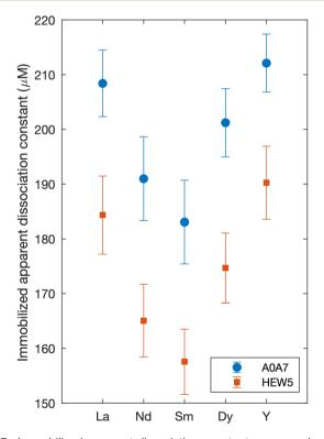
Fig. 7 Immobilized apparent dissociation constants measured under isocratic elution conditions (pH 3) for A0A7 and HEW5. The error bars represent the propagated standard deviations from three independent trials. The uncertainties stem from the experimentally determined capacity ( $B_{\rm t}$ ) and the standard deviations from the retention peaks ( $V_{\rm R}$ ) of each element. Triplicate measurements of apparent dissociation constants and elution profiles are presented in ESI (Fig. S19†).
