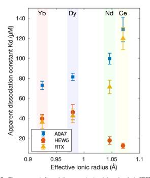
Fig. 3 The apparent dissociation constants, determined *via* FRET, as a function of the effective ionic radius for the three most selective domains (A0A7, HEW5, and RTX). The error bars represent 95% confidence intervals.
