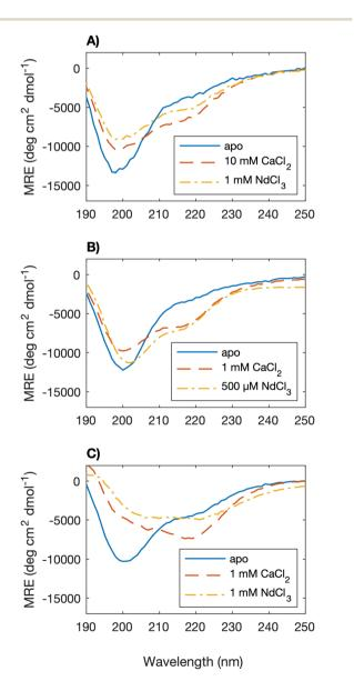
Fig. 4 CD spectra of the proteins (60  $\mu$ M) in their apo (—), Ca-bound (— —), and Nd-bound (— -) states for (A) A0A7, (B) HEW5, and (C) RTX. The reported spectra are the means of three scans.
