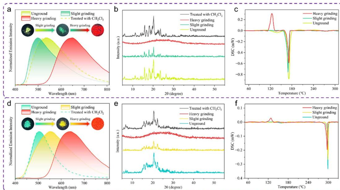
Fig. 2 Normalized PL spectra and PL photographs under 365 nm UV light of the as-synthesized, slightly ground, and heavily ground solid states of **Sym-*m*-OMe** (a), **Sym-*p*-OMe** (d). PXR patterns of **Sym-*m*-OMe** (b) and **Sym-*p*-OMe** (e) in various solid states. DSC curves of **Sym-*m*-OMe** (c) and **Sym-*p*-OMe** (f) in various solid states. The scan rate is 5 °C min<sup>-1</sup> under N<sub>2</sub>.
