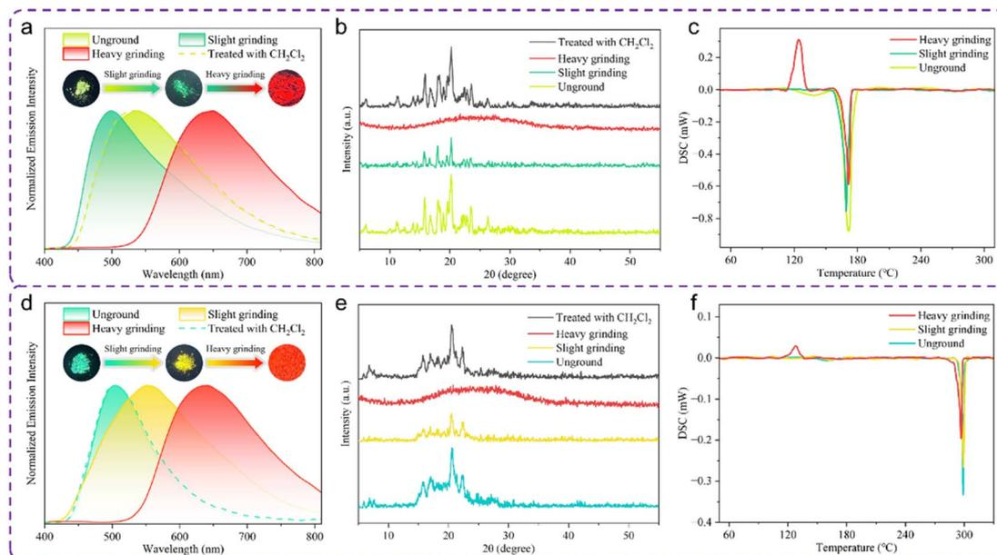
Fig. 2 Normalized PL spectra and PL photographs under 365 nm UV light of the as-synthesized, slightly ground, and heavily ground solid states of **Sym-*m*-OMe** (a), **Sym-*p*-OMe** (d). PXRD patterns of **Sym-*m*-OMe** (b) and **Sym-*p*-OMe** (e) in various solid states. DSC curves of **Sym-*m*-OMe** (c) and **Sym-*p*-OMe** (f) in various solid states. The scan rate is 5 °C min<sup>-1</sup> under N<sub>2</sub>.
