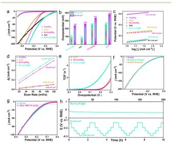
Fig. 3 (a) LSV curves and (b)  $\eta_{10}$  and  $\eta_{50}$  values for Ru-Co<sub>x</sub>Pv@C and reference samples. (c) Corresponding Tafel plots for Ru-Co<sub>x</sub>Pv@C and reference samples. (d)  $C_{\rm dl}$  values for different catalysts (e) TOF values. (f) LSV for Ru-Co<sub>x</sub>Pv@C in various solutions. (g) Polarization curves for the HER after 1000 cycles. (h) Chronopotentiometric curves and multi-step chronopotentiometry test results for Ru-Co<sub>x</sub>Pv@C.
