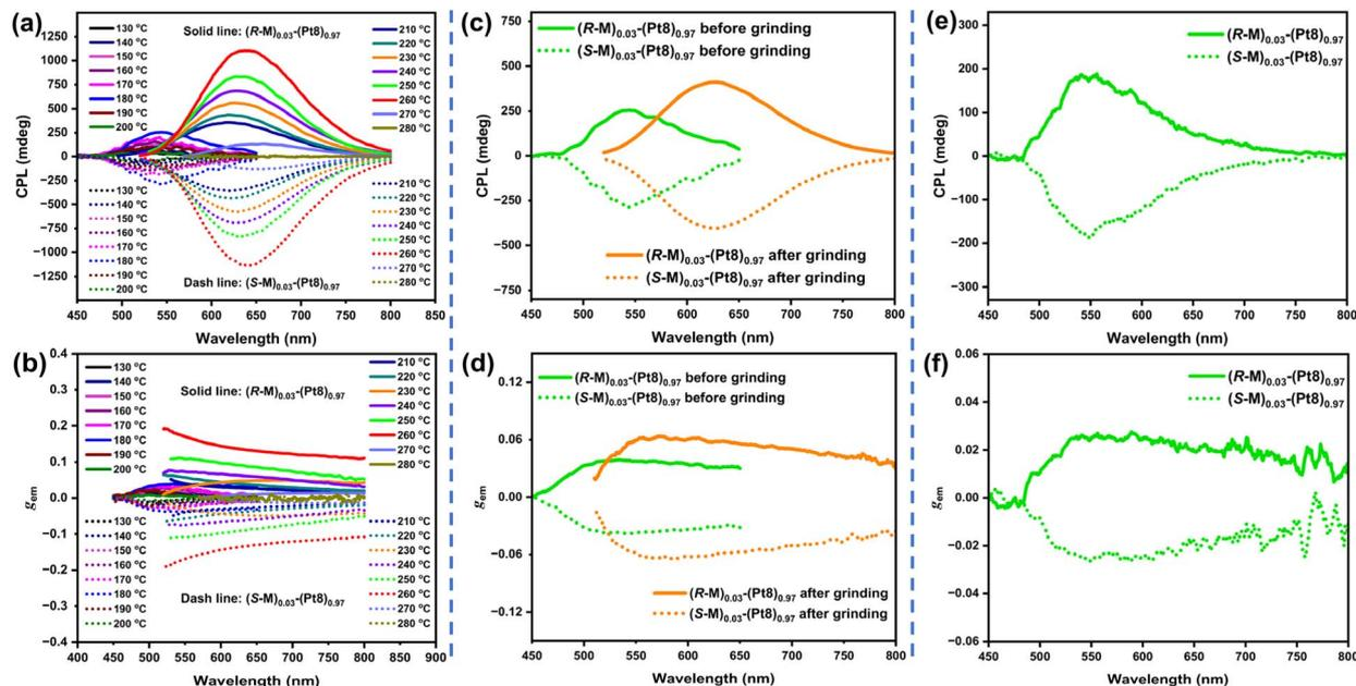
Fig. 4 Temperature-responsive CPL spectra (a) and  $g_{em}$  values vs. wavelength (b) of  $(R/S-M)_{0.03}-(Pt8)_{0.97}$ ; mechanically-responsive CPL spectra (c) and  $g_{em}$  values vs. wavelength (d) of 180 °C-annealed  $(R/S-M)_{0.03}-(Pt8)_{0.97}$  before and after mechanical grinding; recovered CPL spectra (e) and  $g_{em}$  values vs. wavelength (f) of the grinding films  $(R/S-M)_{0.03}-(Pt8)_{0.97}$  after reheating to 180 °C.
