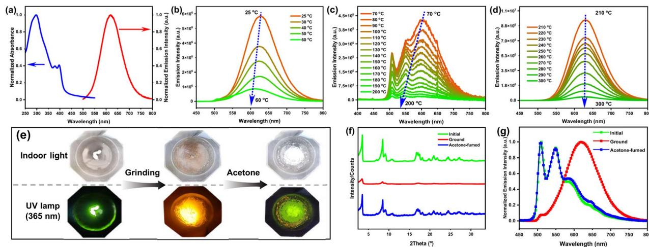
Fig. 1 Ultraviolet-visible (UV-vis) absorption and PL spectra of Pt8 in a spin-coated film ( $6 \text{ mg mL}^{-1}$  in chloroform; 1000 rpm, 30 s) at room temperature (a); PL spectra of Pt8 after thermal annealing at different temperatures (b–d); the photos (e), XRD patterns (f) and PL switching (g) of Pt8 at the initial powder, ground and acetone fumigation states.
