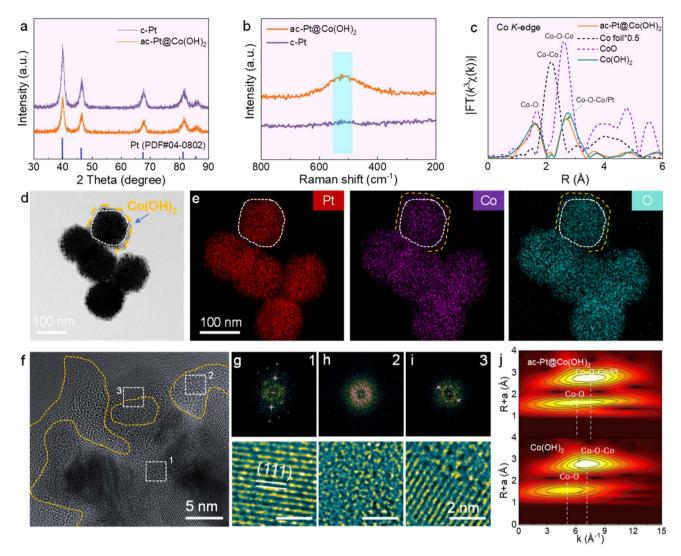
Fig. 1 (a) XRD patterns and (b) Raman patterns of c-Pt and ac-Pt@Co(OH)<sub>2</sub>. (c) EXAFS spectra at the Co K-edge. (d) TEM, (e) EDX element mappings, and (f) HRTEM images of ac-Pt@Co(OH)<sub>2</sub>. (q-i) FFT and corresponding IFFT patterns of the selected regions in (f). (j) WT for the Co k<sup>5</sup>weighted EXAFS signal of Co(OH)2 and ac-Pt@Co(OH)2.
