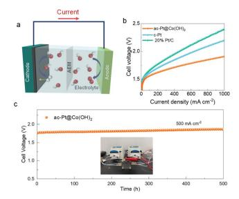
Fig. 5 (a) Schematic diagram of a membrane-electrode-assembly (MEA)-based AEMWE device. (b) Polarization curves of the AEMWE using ac-Pt@Co(OH)<sub>2</sub>, c-Pt, and Pt/C. (c) Durability test of the ac-Pt@Co(OH)<sub>2</sub>-based AEM electrolyser at a current density of 500 mA cm<sup>-2</sup>. Insets show the photographs of the AEMWE device.
