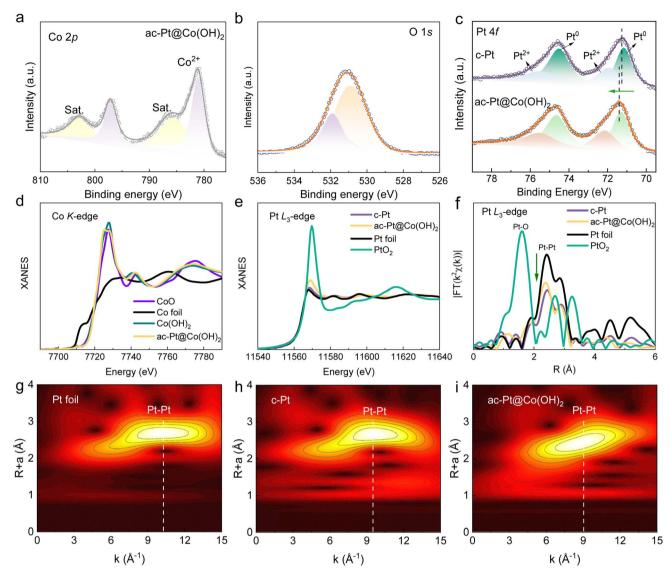
Fig. 2 (a) Co 2p and (b) O 1s XPS spectra of ac-Pt@Co(OH)<sub>2</sub>. (c) Pt 4f XPS spectra of ac-Pt@Co(OH)<sub>2</sub> and c-Pt. (d and e) Co K-edge and Pt L<sub>3</sub>-edge XANES spectra. (f) EXAFS spectra at the Pt L<sub>3</sub>-edge. (g-i) WT-EXAFS plots of the Pt L<sub>3</sub>-edge for Pt foil, c-Pt, and ac-Pt@Co(OH)<sub>2</sub>.
