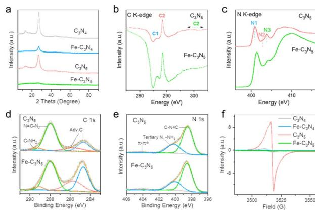
Fig. 2 Structural characterization of catalysts. (a) XRD patterns of  $C_3N_4$ ,  $C_3N_5$ , Fe- $C_3N_4$ , and Fe- $C_3N_5$ . (b) C K-edge NEXAFS of  $C_3N_5$  and Fe- $C_3N_5$ . (c) N K-edge X-ray NEXAFS of  $C_3N_5$  and Fe- $C_3N_5$ . (d) C 1s XPS spectra of  $C_3N_5$  and Fe- $C_3N_5$ . (e) N 1s XPS spectra of  $C_3N_5$  and Fe- $C_3N_5$ . (f) EPR spectra of  $C_3N_4$ ,  $C_3N_5$ , Fe- $C_3N_4$ , and Fe- $C_3N_5$ .
