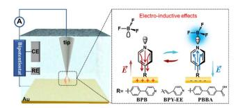
Scheme 1 Schematic diagram of STM-BJ methods used to probe the electro-induced effect of the  $N-BF_3$  Lewis bond in LiBF<sub>4</sub> solution, which can regulate metal-molecule contacts in the single-molecule junction for switching.
