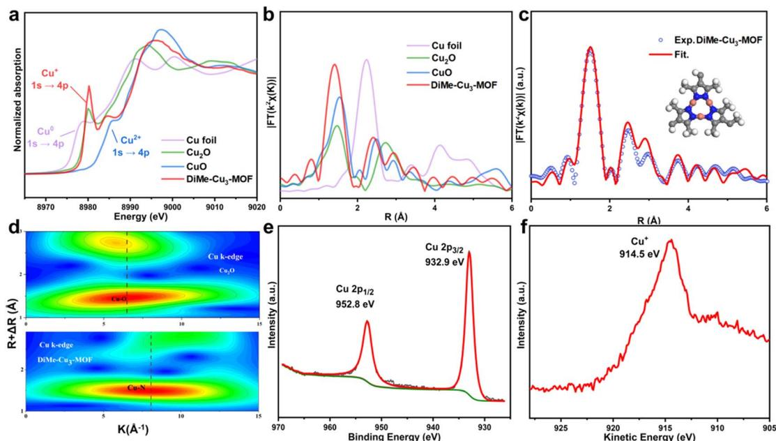
Fig. 3 (a) Cu K-edge of XANES spectra of DiMe-Cu<sub>3</sub>-MOF, Cu foil, CuO and Cu<sub>2</sub>O. (b) Cu K-edge of EXAFS spectra of DiMe-Cu<sub>3</sub>-MOF, Cu foil, CuO and Cu<sub>2</sub>O. (c) The EXAFS fitting curves of DiMe-Cu<sub>3</sub>-MOF. (d) WT-EXAFS plots of DiMe-Cu<sub>3</sub>-MOF and Cu<sub>2</sub>O. (e) Cu 2p XPS spectra and (f) Cu LMM Auger spectra of DiMe-Cu<sub>3</sub>-MOF.
