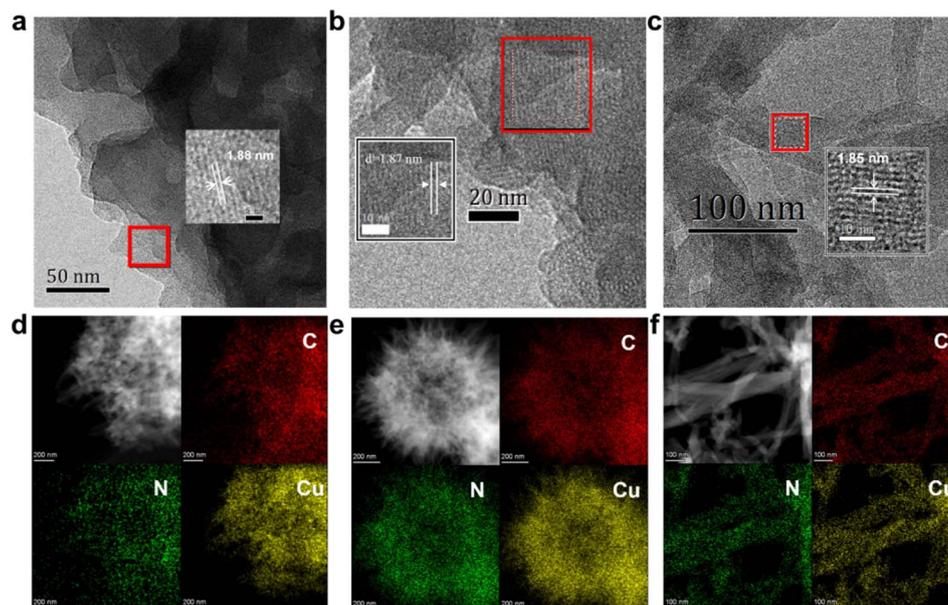
Fig. 2 HR-TEM image and the lattice distance of (a) NonMe-Cu<sub>3</sub>-MOF, (b) UniMe-Cu<sub>3</sub>-MOF and (c) DiMe-Cu<sub>3</sub>-MOF. (d-f) HAADF-STEM image of (d) NonMe-Cu<sub>3</sub>-MOF, (e) UniMe-Cu<sub>3</sub>-MOF and (f) DiMe-Cu<sub>3</sub>-MOF and the corresponding C, N, and Cu EDS elemental mappings.
