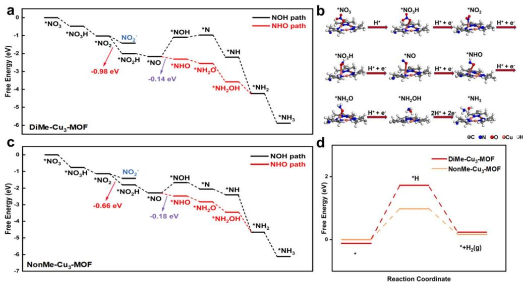
Fig. 6 (a) Gibbs free energy diagram for the NO<sub>3</sub>RR on DiMe-Cu<sub>3</sub>-MOF. (b) The most probable pathway of the NO<sub>3</sub>RR on DiMe-Cu<sub>3</sub>-MOF (side view). (c) Gibbs free energy diagram for the NO<sub>3</sub>RR on NonMe-Cu<sub>3</sub>-MOF. (d) Gibbs free energy diagram for the HER on DiMe-Cu<sub>3</sub>-MOF and NonMe-Cu<sub>3</sub>-MOF.
