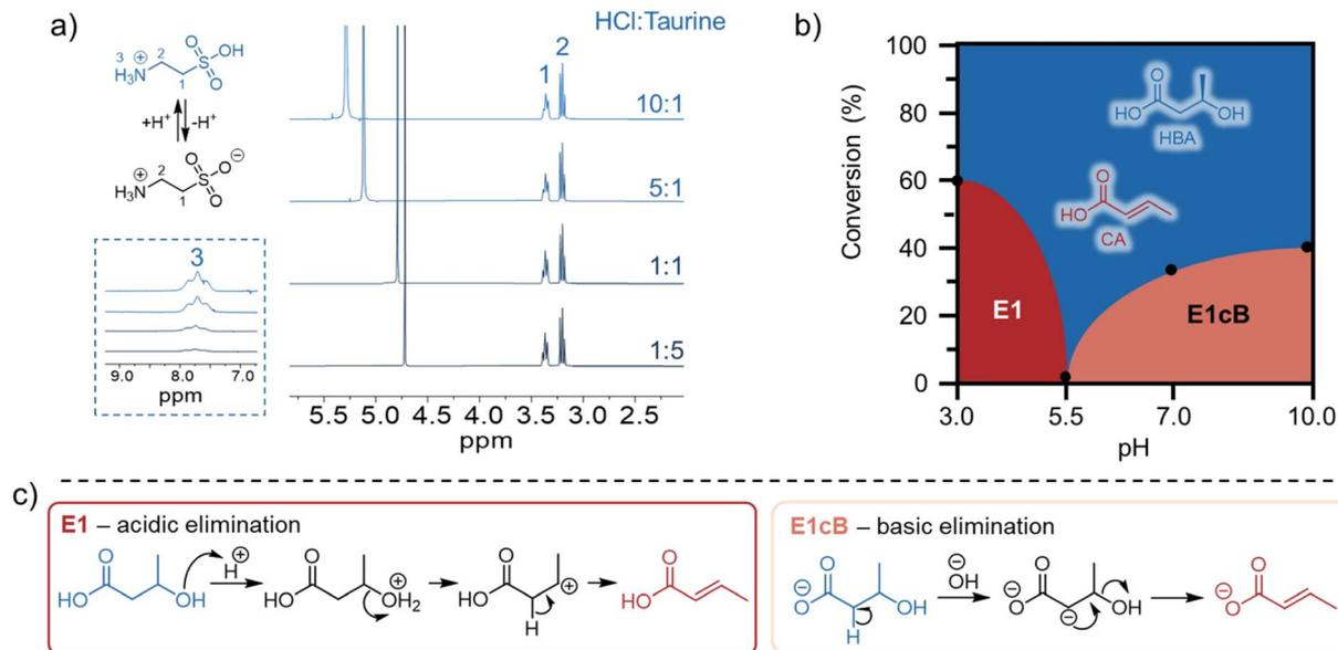
Fig. 3 (a) <sup>1</sup>H NMR study of the taurine structure with different equivalents of HCl. (b) The influence of pH on the HBA/CA ratio (black dots represent experimental points). (c) The proposed mechanism of elimination in acidic or basic media.
