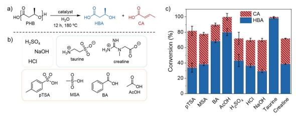
Fig. 2 (a) PHB hydrolytic depolymerization to give HBA and CA. (b) Catalysts employed in the screening process. (c) Conversion of PHB and relative selectivity for HBA and CA formation.
