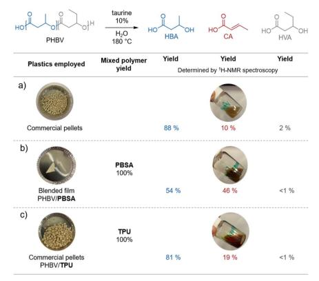
Fig. 5 Depolymerization process of commercial PHB-based samples (a) PHBV, (b) PHBV + PBSA and (c) PHBV + TPU.
