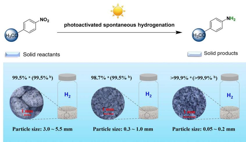
Fig. 2 Catalytic evaluation of solid reactants under different particle size distributions: <sup>a</sup>HPLC yield of the whole reaction system; <sup>b</sup>chemoselectivity.
