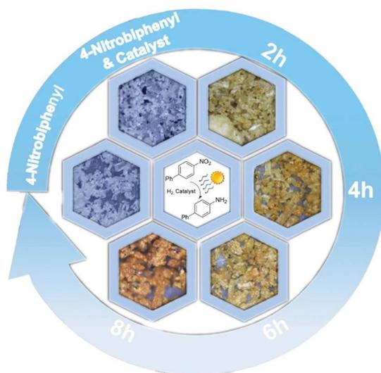
Fig. 6 Monitoring the reaction progress by optical microscopy. The physical form of **1e** in the reaction dramatically changes from a highly aggregated crystal structure to a plastic-like appearance during the reaction.
