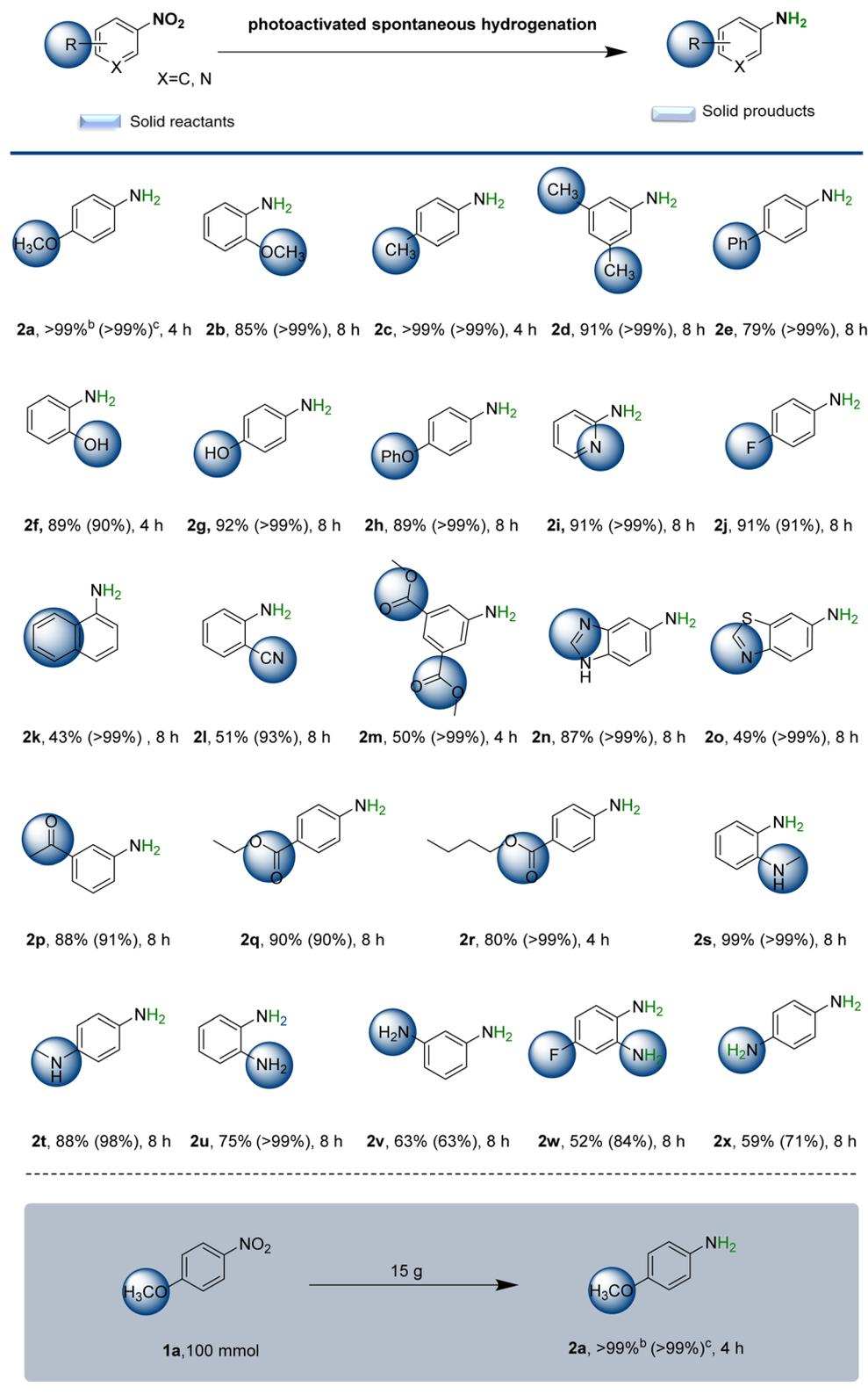
Scheme 2 Solar-driven and spontaneous solid-state synthesis of functionalized nitro compounds over 12R-Pd-NCs. <sup>a</sup>Catalytic conditions unless otherwise noted: 0.5 mmol of solid-state nitro compound, 12R-Pd-NCs (2 mg), H<sub>2</sub> balloon (1 atm), illuminate for 4 hours under sunlight, or a 100 W xenon lamp/tungsten filament lamp; <sup>b</sup>HPLC yield of the whole reaction system; <sup>c</sup>chemoselectivity.
