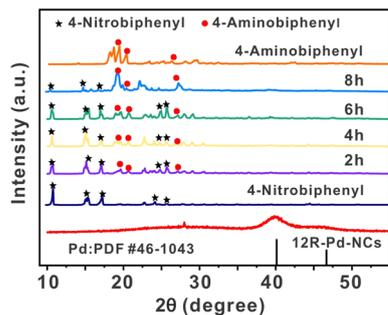
Fig. 5 Monitoring the reaction progress by PXRD analysis.
