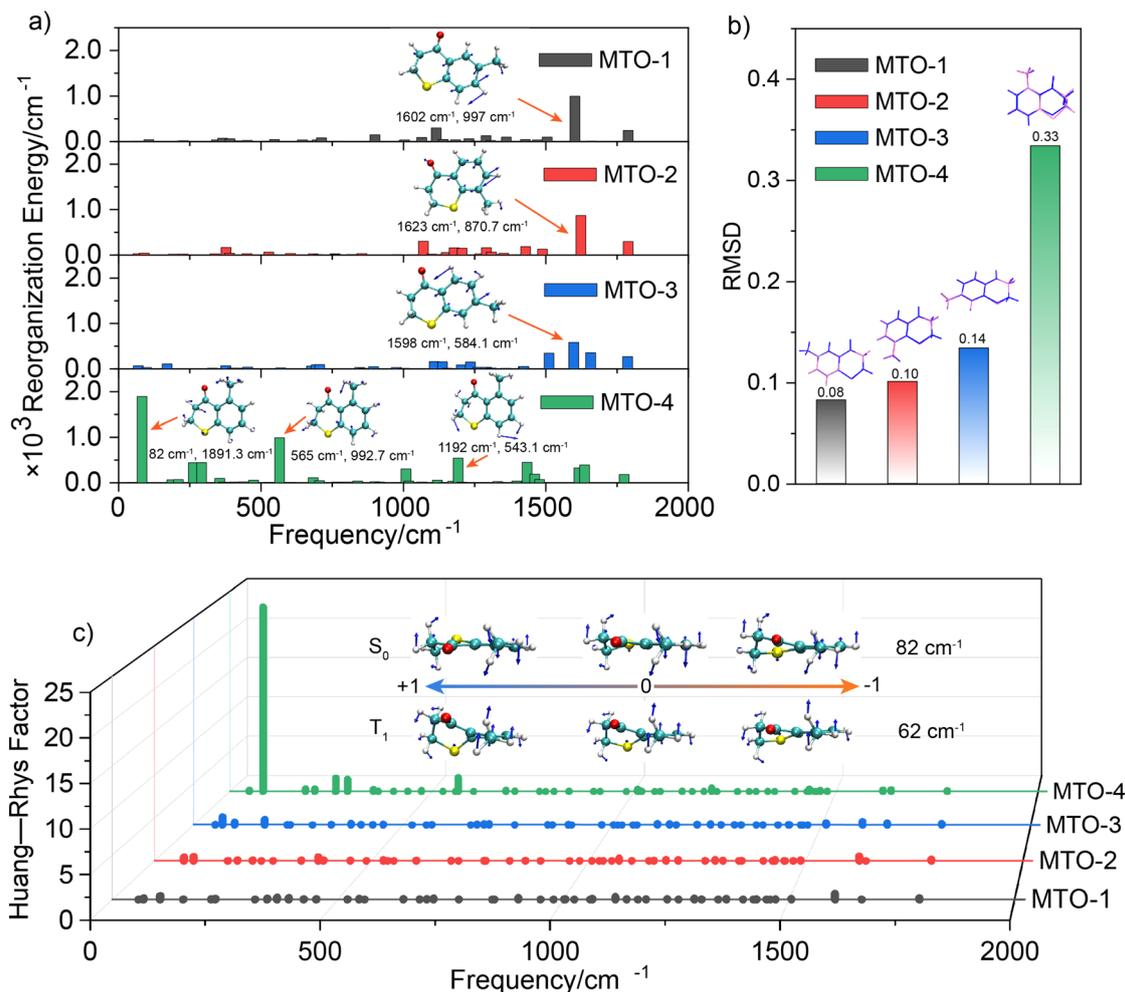
Fig. 4 (a) Calculated reorganization energies of the  $T_1 \rightarrow S_0$  transition are plotted against the frequencies of MTOs. Representative high-intensity (>500  $\text{cm}^{-1}$ ) vibration modes are shown as insets; (b) schematic distribution of RMSD  $T_0 \rightarrow S_0$  values; (c) Huang-Rhys factors of MTOs from  $T_1$  to  $S_0$ . The insets show the most representative intramolecular vibration modes of MTO-4 in  $S_0$  and  $T_1$  states.
