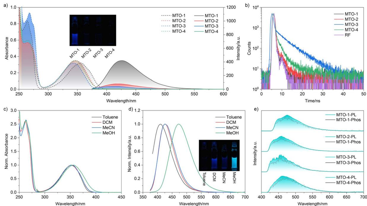
Fig. 1 a) Absorption and emission spectra of MTOs in DCM; (b) lifetime spectra of MTOs in DCM; absorption (c) and emission (d) spectra of MTO-1 in different solvents; (e) steady-state and phosphorescence spectra of MTOs in MTHF at 77 K.
