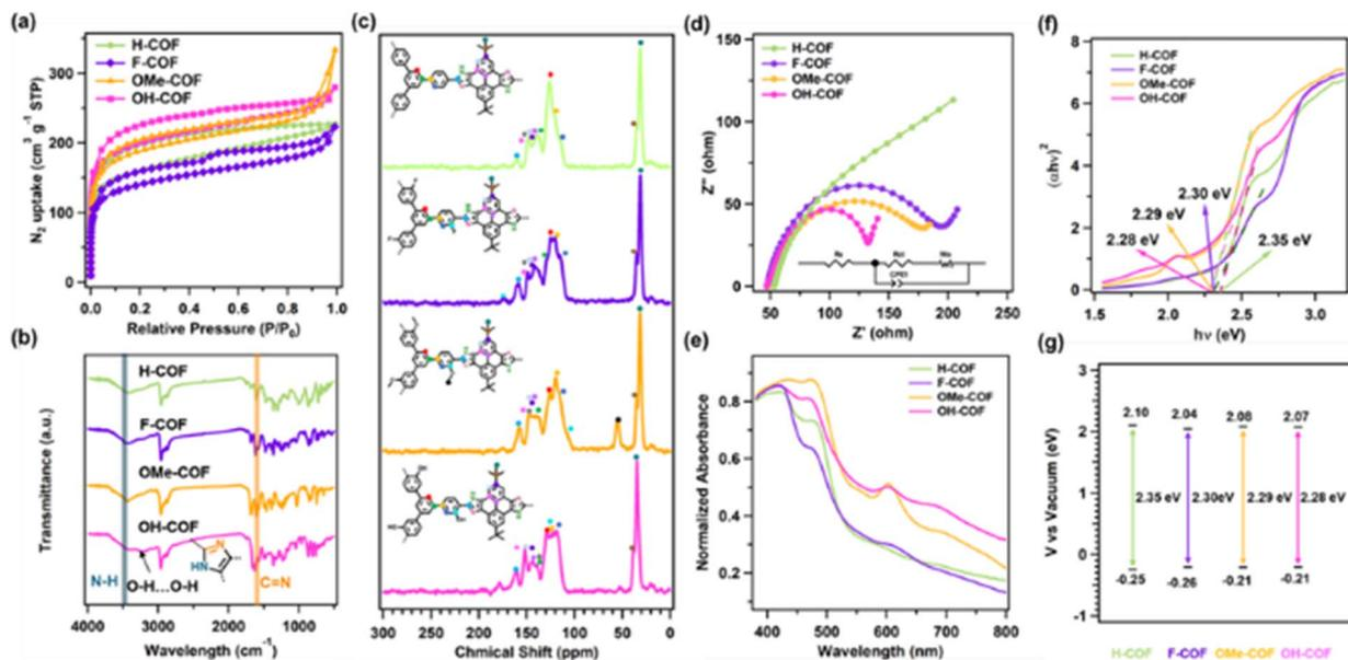
Fig. 2 Structural characterization, EIS and UV/vis spectroscopy spectra of H-COF, F-COF, OMe-COF and OH-COF. (a) Nitrogen sorption isotherm curves. (b) FT-IR curves. (c) The  $^{13}\text{C}$  NMR spectra, (d) Nyquist plots of electrochemical impedance spectroscopy (EIS), (e) UV/Visible diffuse reflectance plots, (f) Tauc plots and (g) LUMO and HOMO levels of H-COF (green), F-COF (purple), OMe-COF (orange) and OH-COF (pink), respectively.
