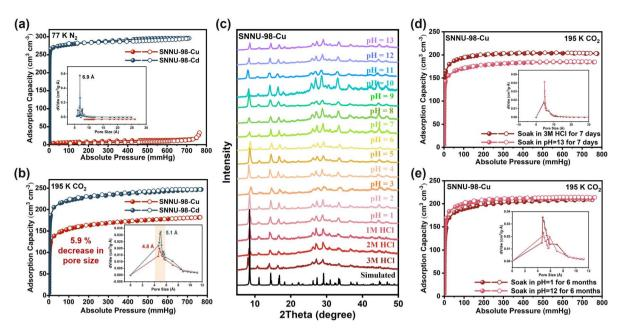
Fig. 2 Stability and porosity of SNNU-98-Cd/Cu MOFs: (a) 77 K  $N_2$  adsorption and calculated pore size distributions; (b) 195 K  $CO_2$  adsorption and calculated pore size distributions; (c) PXRD patterns of SNNU-98-Cu immersed in pH -0.5-13 solution for 1 week; (d and e) 195 K  $CO_2$  adsorption curves and calculated pore size distributions of SNNU-98-Cu after immersion in -0.5-13 solution for 1 week and pH 1-12 solution for 6 months
