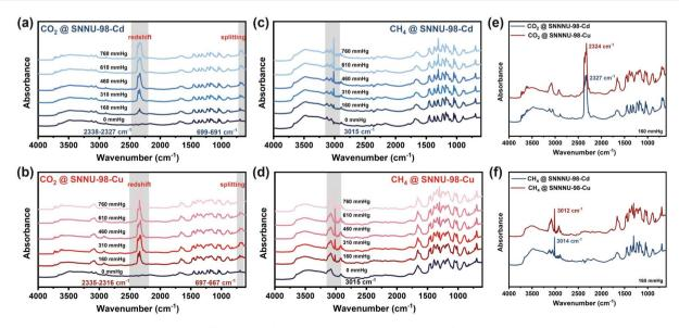
Fig. 5 In situ FT-IR spectra for SNNU-98-Cd/Cu: (a and b) for the CO<sub>2</sub> adsorption process; (c and d) for the CH<sub>4</sub> adsorption process; (e and f) comparison of CO<sub>2</sub> and CH<sub>4</sub> adsorption.
