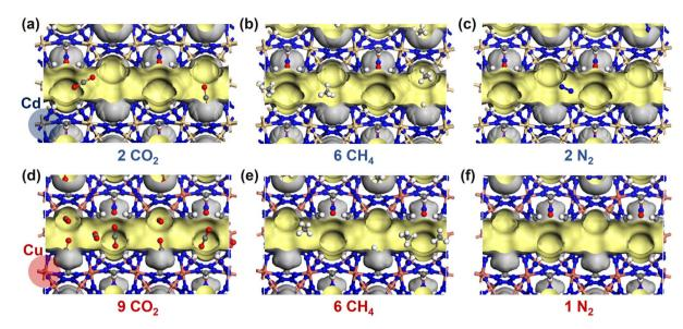
Fig. 6 GCMC-simulated (a and d) CO<sub>2</sub>, (b and e) CH<sub>4</sub>, and (c and f) N<sub>2</sub> distributions in the channel of SNNU-98-Cd/Cu MOFs.
