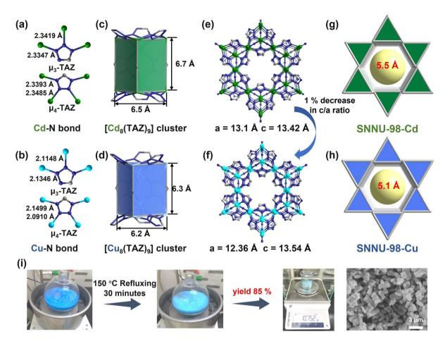
Fig. 1 Illustration of the structures and rapid reflux synthesis route of SNNU-98-Cd/Cu MOFs: (a and b) comparison of metal–N bond lengths; (c and d) detailed comparison of  $[Cd_8(TAZ)_9]$  and  $[Cu_8(TAZ)_9]$  clusters; (e, f, j, and h) detailed comparison of the 3D porous frameworks and 1D hexagonal channel viewed along the c-axis direction; (i) scaled-up production of SNNU-98-Cu material.
