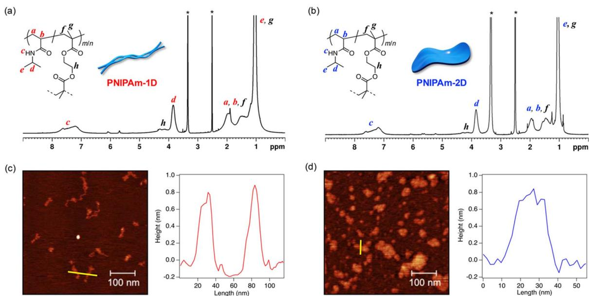
**Fig. 3**  $^1\text{H}$  NMR spectra of (a) **PNIPAm-1D** and (b) **PNIPAm-2D** (cross-linking ratios: 10 and 6 mol%, respectively). AFM images and height profiles of (c) **PNIPAm-1D** and (d) **PNIPAm-2D**. Samples were deposited on a mica substrate by spin-casting dilute  $\text{CHCl}_3$  solutions thereof. The height profiles were recorded along the yellow lines in the corresponding AFM images.
