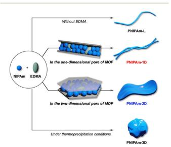
Fig. 1 Schematic illustration of the synthesis of linear PNIPAm (PNI-PAm-L) and PNIPAms with 1D, 2D, and 3D network topologies (PNI-PAm-1D, PNIPAm-2D, and PNIPAm-3D, respectively).
