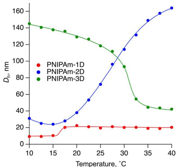
Fig. 5 Hydrodynamic diameters ( $D_h$ ) of PNIPAm-1D (red), PNIPAm-2D (blue), and PNIPAm-3D (green) in aqueous solutions, measured by DLS at different temperatures. The plotted particle sizes correspond to the peak with the highest volume fraction. The volume-based distributions are shown in Fig. S8.†
