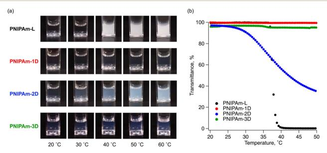
Fig. 4 (a) Appearances of aqueous solutions of PNIPAm at different temperatures. (b) Temperature dependence of the optical transmittance of aqueous solutions of PNIPAm-L (black), PNIPAm-1D (red), PNIPAm-2D (blue), and PNIPAm-3D (green).
