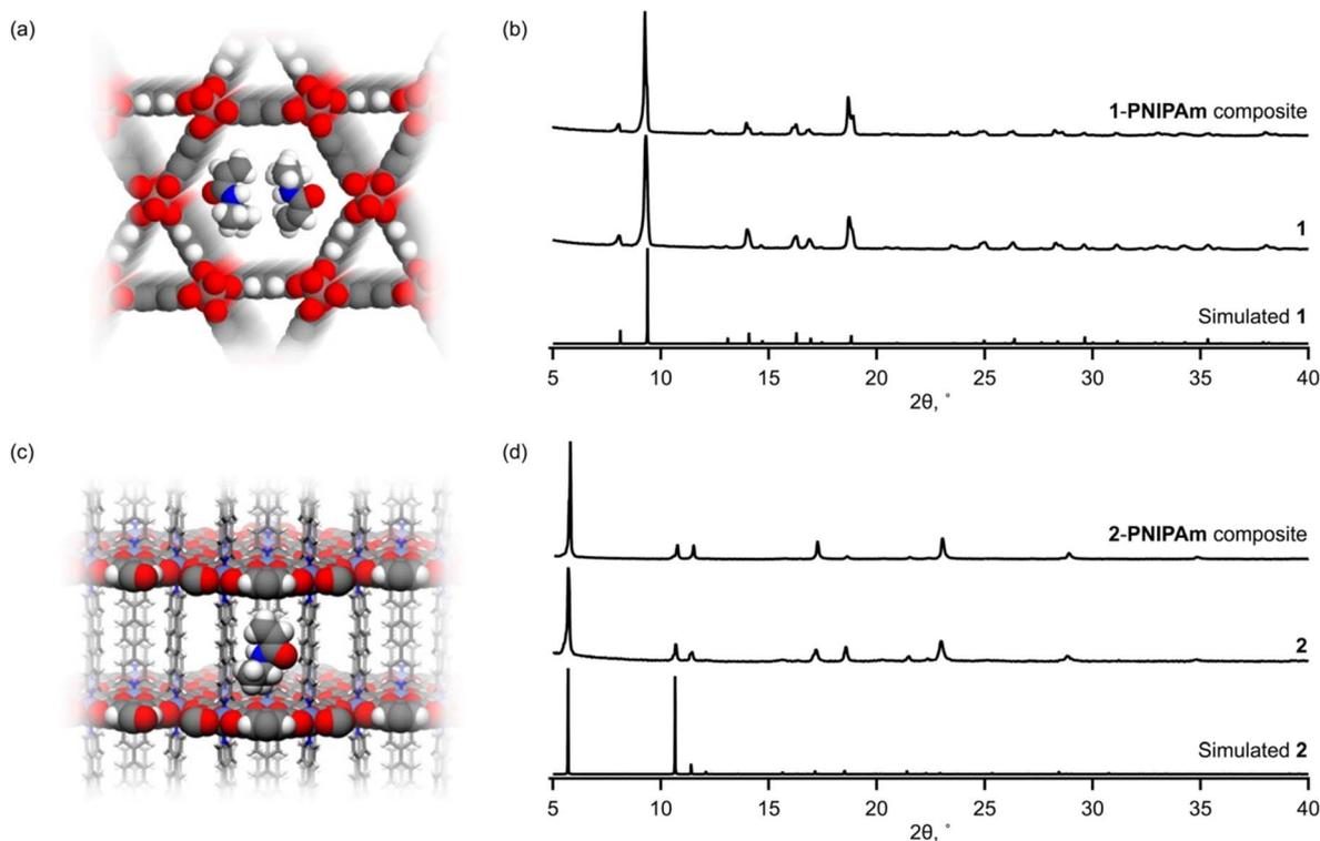
**Fig. 2** (a) Crystal structure of **1**; monomers (NIPAm) were inserted into the cavity by molecular modeling. (b) XRPD patterns of simulated **1**, **1**, and **1**-PNIPAm composite. (c) Crystal structure of **2**; the monomer was inserted into the cavity by molecular modeling. The pillar ligands (dpb) in **2** are shown as stick models for clarity. (d) XRPD patterns of simulated **2**, **2**, and **2**-PNIPAm composite. Atoms: In (brown), Ni (purple), O (red), N (blue), C (gray), H (white).
