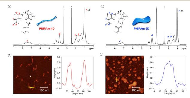
Fig. 3 <sup>1</sup>H NMR spectra of (a) PNIPAm-1D and (b) PNIPAm-2D (cross-linking ratios: 10 and 6 mol%, respectively). AFM images and height profiles of (c) PNIPAm-1D and (d) PNIPAm-2D. Samples were deposited on a mica substrate by spin-casting dilute CHCl<sub>3</sub> solutions thereof. The height profiles were recorded along the yellow lines in the corresponding AFM images.
