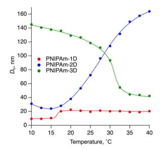
Fig. 5 Hydrodynamic diameters ( $D_{\rm h}$ ) of PNIPAm-1D (red), PNIPAm-2D (blue), and PNIPAm-3D (green) in aqueous solutions, measured by DLS at different temperatures. The plotted particle sizes correspond to the peak with the highest volume fraction. The volume-based distributions are shown in Fig. S8.†
