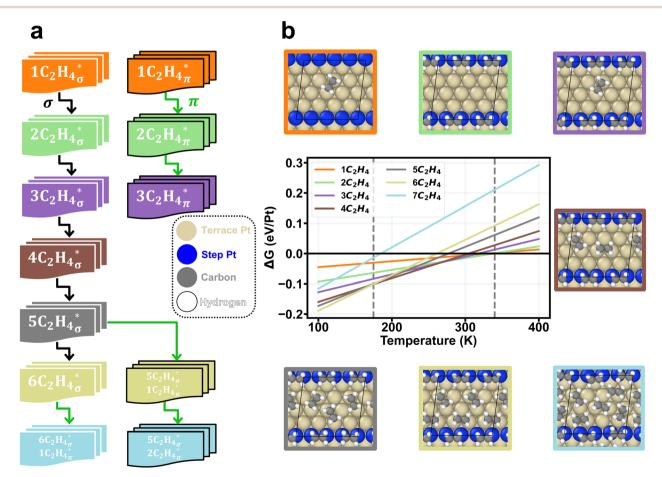
Fig. 5 Coverage-dependent phase diagram of ethylene adsorption on Pt(553). (a) Workflow to achieve the seven coverages. (b) Coveragedependent phase diagram of ethylene adsorbed on Pt(553) surface. The adsorption free energy is plotted as a function of the surface temperature. Snapshots of the most stable configurations at different coverages are shown. The dashed vertical lines mark the calculated lower and upper limits of the desorption temperature range
