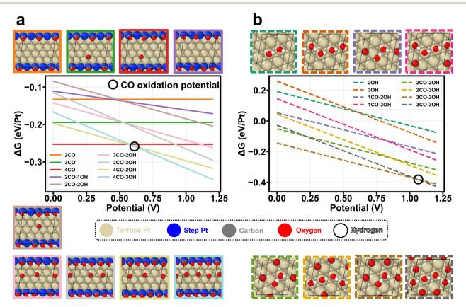
Fig. 4 Coverage-dependent phase diagram of CO\*-OH\* co-adsorption on (a) Pt(553) and (b) Pt(111) surfaces. The adsorption free energy is plotted as a function of the applied potential relative to the standard hydrogen electrode (SHE). Top-view snapshots of the most stable configurations under all coverages are shown. Estimated CO\* oxidation potentials on both surfaces are marked by black circles.
