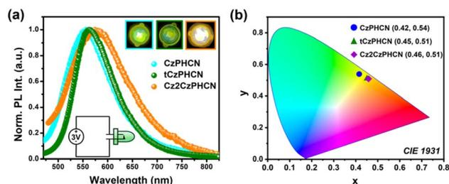
Fig. 5 (a) Emission spectrum of all three emitter-fabricated c-LEDs. (b) Chromaticity plots (CIE 1931) of all emitters.
