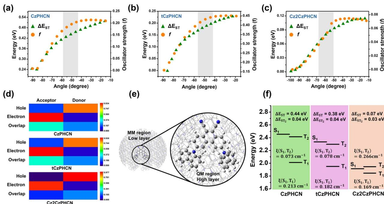
Fig. 1 Plot of  $\Delta E_{ST}$  and oscillator strength vs. dihedral angle ( $\theta_{DA}$ ) of (a) *Cz*PHCN, (b) *tCz*PHCN and (c) *Cz2Cz*PHCN. (d) The heat maps of the distribution of electron–hole in the donor and acceptor moiety in the  $S_1$  state. (e) High layer (QM region) and low layer (MM region) from the crystal structure for QM/MM calculation. (f) Single point energies and spin–orbit coupling (SOC) from TD-DFT calculation based on QM/MM calculation.
