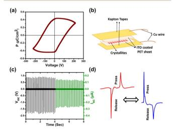
Fig. 6 (a) P-E hysteresis loop for CzPHCN. (b) Schematic showing the fabrication of a piezoelectric nanogenerator device. (c) Open circuit peak-to-peak voltage ( $V_{PP}$ ) and calculated short-circuit current ( $I_{PP}$ ) of as-made piezo device (the shifted time axis provided here is a guide to the eye). (d) Peak-to-peak voltage profiles for a single cycle of signals in the forward and reverse polarity connections.
