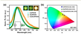
Fig. 5 (a) Emission spectrum of all three emitter-fabricated c-LEDs. (b) Chromaticity plots (CIE 1931) of all emitters.
