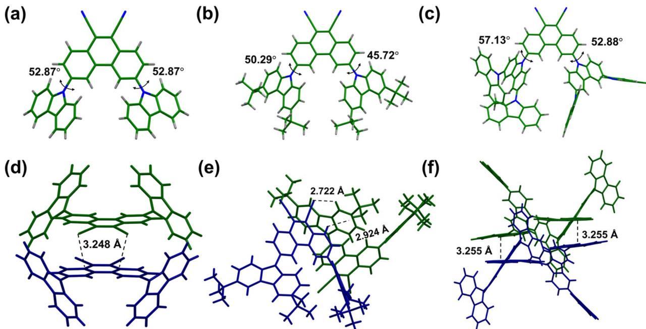
Fig. 2 Crystal structure of (a) CzPHCN, (b) *t*CzPHCN and (c) Cz2CzPHCN with the donor–acceptor dihedral angle ( $\theta_{DA}$ ). Crystal packing interaction of (d) CzPHCN, (e) *t*CzPHCN and (f) Cz2CzPHCN.
