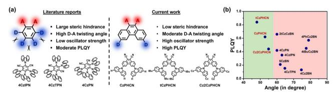
Scheme 1 (a) Molecular designing principle: chemical structure of 4CzIPN, 4CzTPN and 4CzPN from the literature report (left),¹ chemical structure of CzPHCN, tCzPHCN and Cz2CzPHCN investigated in this work (right). (b) PLQY vs. dihedral angle plot of carbazole-based molecules reported in the literature, and the molecules in this work (see ESI Section S12†).
