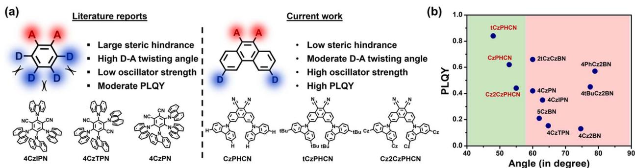
Scheme 1 (a) Molecular designing principle: chemical structure of 4CzIPN, 4CzTPN and 4CzPN from the literature report (left),<sup>1</sup> chemical structure of CzPHCN, tCzPHCN and Cz2CzPHCN investigated in this work (right). (b) PLQY vs. dihedral angle plot of carbazole-based molecules reported in the literature, and the molecules in this work (see ESI Section S12†).
