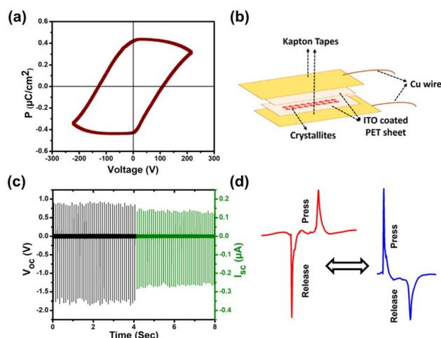
Fig. 6 (a)  $P$ - $E$  hysteresis loop for CzPHCN. (b) Schematic showing the fabrication of a piezoelectric nanogenerator device. (c) Open circuit peak-to-peak voltage ( $V_{pp}$ ) and calculated short-circuit current ( $I_{sc}$ ) of as-made piezo device (the shifted time axis provided here is a guide to the eye). (d) Peak-to-peak voltage profiles for a single cycle of signals in the forward and reverse polarity connections.
