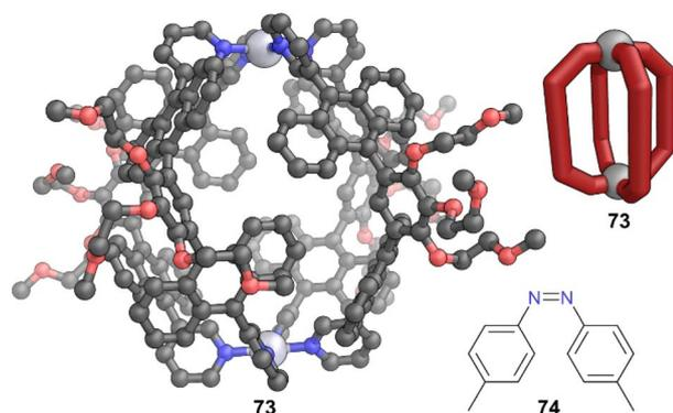
Fig. 20 Representation of the SCXRD structure of cage 73, which selectively encapsulates the *cis*-form of azobenzene 74. Disorder, solvent, hydrogen atoms, and counter anions have been omitted for clarity. Colour: C = grey, N = blue, O = red, Pt = light grey.
