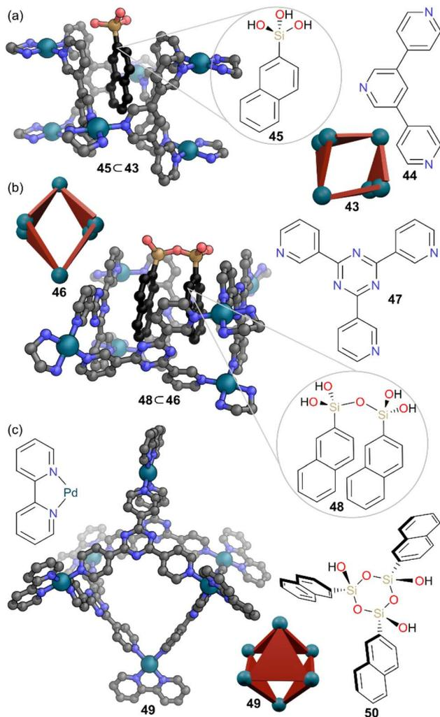
Fig. 13 (a) Representation of the SCXRD structure of  $45 \subset 43$ , showing the encapsulation of 'monomeric' silanetriol 45. (b) Representation of the SCXRD structure of  $48 \subset 46$ , showing the encapsulation of silanol dimer 48. (c) Representation of the SCXRD structure of 49 which encapsulates silanol cyclic trimer 50. Disorder, solvent, hydrogen atoms, and counter anions have been omitted for clarity. Colour: C = grey or black, N = blue, O = red, Pd = turquoise, Si = sand.
