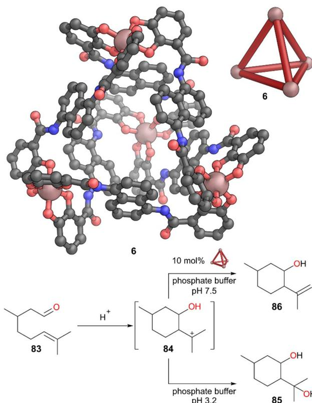
Fig. 23 Representation of the SCXRD structure of cage **6** and selective reaction of citronellal **83** to alkene **86** in presence of cage **6**. Disorder, solvent, hydrogen atoms, and counter cations have been omitted for clarity. Colour: C = grey, N = blue, O = red, Ga = burnt pink.
