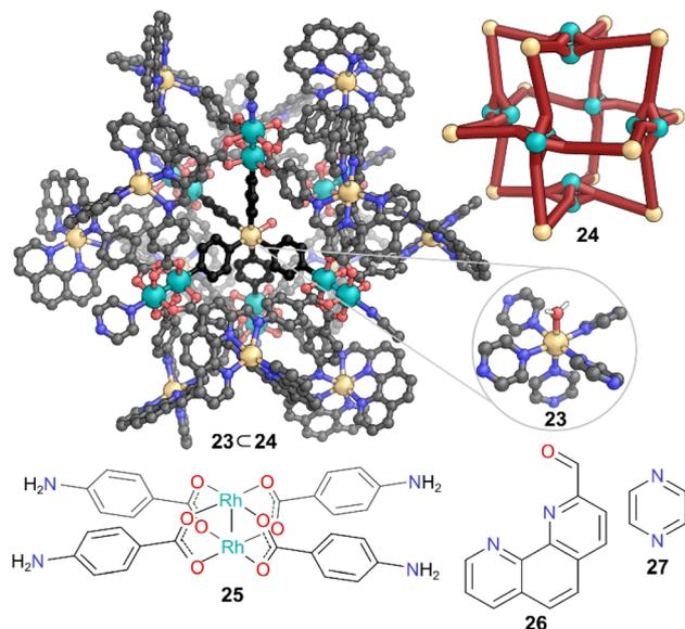
Fig. 7 Representation of the SCXRD structure of  $23 \subset 24$ . Cage  $24$  is constructed from components  $25$  and  $26$ . Disorder, solvent, hydrogen atoms, and counter anions have been omitted for clarity. Colour: C = grey or black, N = blue, O = red, Rh = teal, Cd = light orange.
