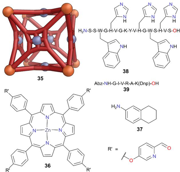
Fig. 11 Cartoon representation of cage **35**, constructed from components **36** and **37**, which binds peptide **38** through the histidines but not peptide **39**. Colour: Zn = cool grey, Fe = orange. Peptides are shown by their standard one letter abbreviation for amino acid residues: A = alanine, G = glycine, H = histidine, I = isoleucine, K = lysine, R = arginine, S = serine, V = valine, W = tryptophan, Y = tyrosine. Abz = 2-aminobenzoyl, Dnp = 2,4-dinitrophenyl.
