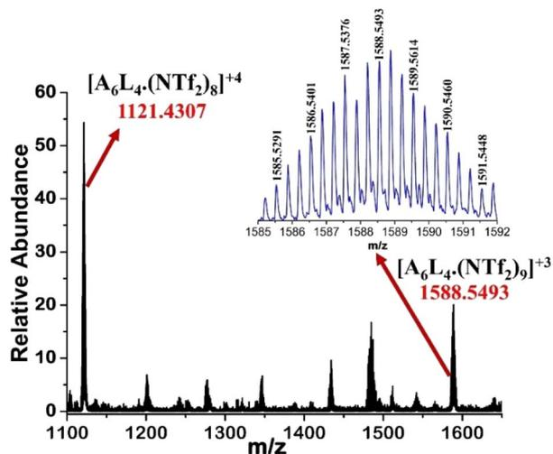
Fig. 2 ESI-MS spectrum of the  $\text{NTf}_2^-$  analogue of **1** in acetonitrile. The experimental isotopic distribution pattern of the  $[\text{A}_6\text{L}_4(\text{NTf}_2)_9]^{3+}$  fragment (inset).
