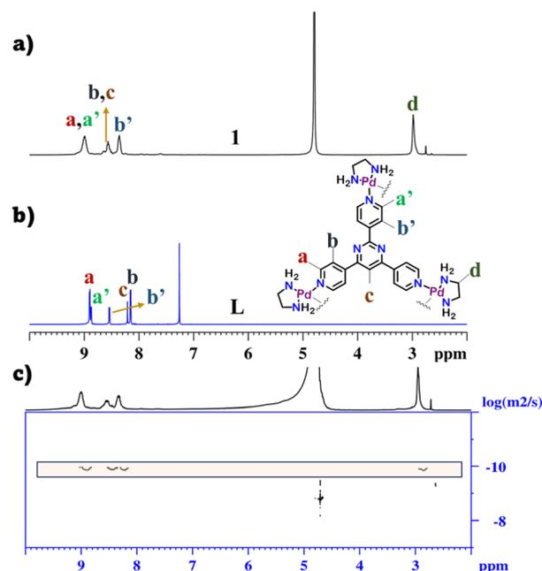
Fig. 1 Stacked <sup>1</sup>H NMR spectra of (a) cage **1** in D<sub>2</sub>O and (b) ligand **L** in CDCl<sub>3</sub>, and (c) <sup>1</sup>H NMR DOSY spectrum of **1** in D<sub>2</sub>O.
