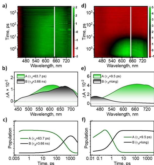
Fig. 3 (a) Femtosecond transient absorption (fsTA) contour plot of HD in THF (colour scale of the contour plot represents  $\Delta A/10^2$  a.u.), (b) deconvoluted EAS plot of HD in THF, (c) deconvoluted decay time constants of the EAS for HD in THF; (d) fsTA contour plot of BrD in THF, (e) deconvoluted EAS plot of BrD in THF, (f) deconvoluted decay time constants of the EAS for BrD in THF.
