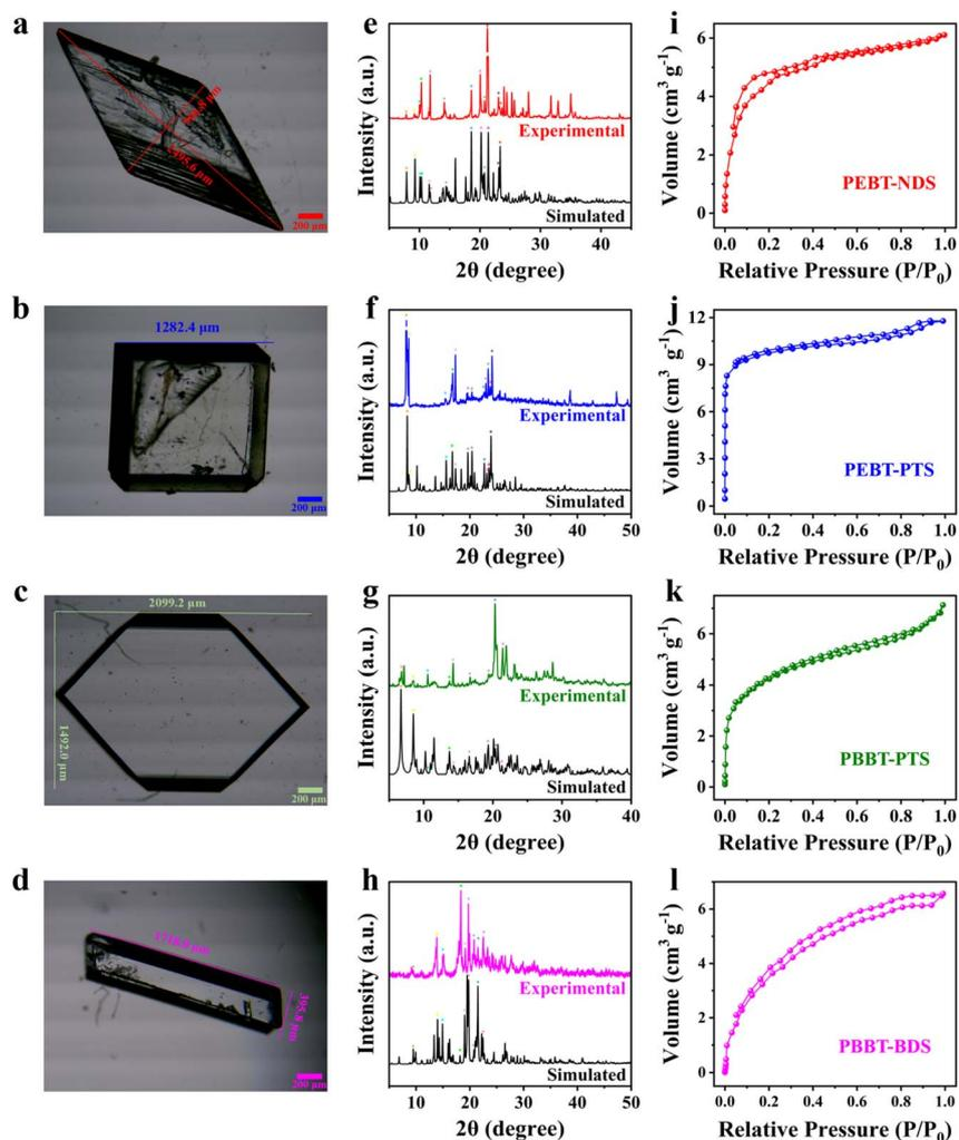
Fig. 2 Optical microscope photographs (a–d), XRD (e–h), and BET specific surface areas (i–l) of PEBT-NDS (a, e and i), PEBT-PTS (b, f and j), PBBT-PTS (c, g and k) and PBBT-BDS (d, h and l).
