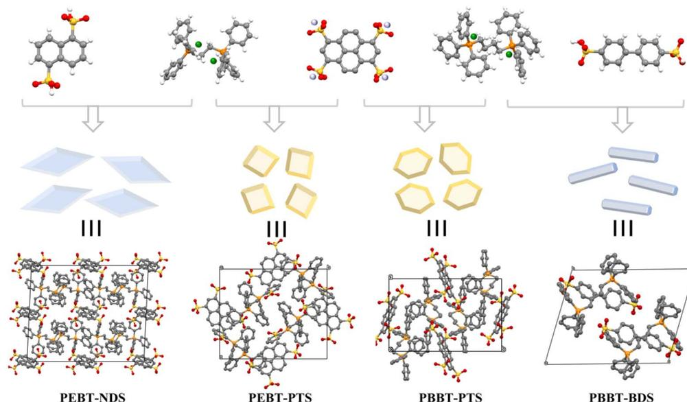
Scheme 1 Synthesis of four IOCs via pair-to-pair ionic self-assembly at room temperature in MeOH/H<sub>2</sub>O.
