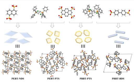
Scheme 1 Synthesis of four IOCs via pair-to-pair ionic self-assembly at room temperature in MeOH/H<sub>2</sub>O.
