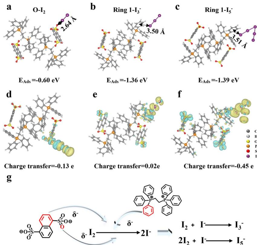
Fig. 6 Adsorption energies and distances of (a)  $O-I_2$ , (b) ring  $1-I_3^-$ , and (c) ring  $1-I_5^-$ , and corresponding charge transfer diagrams (d–f), and (g) formation mechanism of polyiodide anions.
