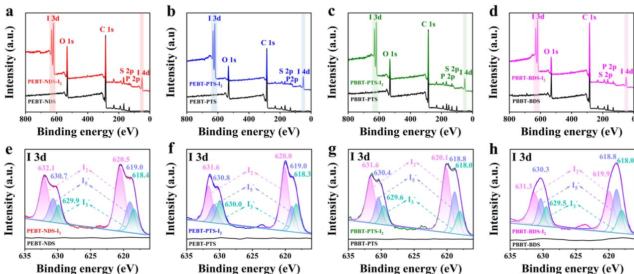
Fig. 4 The XPS full spectrum of the four IOCs before and after iodine adsorption of (a) PEPT-NDS, (b) PEPT-PTS, (c) PBBT-PTS, and (d) PBBT-BDS and the corresponding I 3d high-resolution spectrum (e–h).
