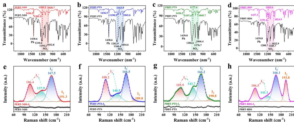
Fig. 5 FT-IR spectrum of the four IOCs before and after iodine adsorption of (a) PEBT-NDS, (b) PEBT-PTS, (c) PBBT-PTS, and (d) PBBT-BDS and the corresponding Raman spectrum (e–h).
