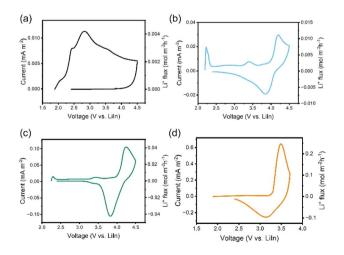
$\label{eq:fig.1} \begin{tabular}{ll} Fig. 1 & The CV curves of (a) LPSCl-VGCF|LPSCl|LiIn, (b) uncoated LNMO-LPSCl-VGCF|LPSCl|LiIn, (c) LTaP@LNMO-LPSCl-VGCF|LPSCl|LiIn and (d) LCO-LPSCl-VGCF|LPSCl|LiIn cells, respectively. The battery used for measurement is newly assembled. \end{tabular}$
