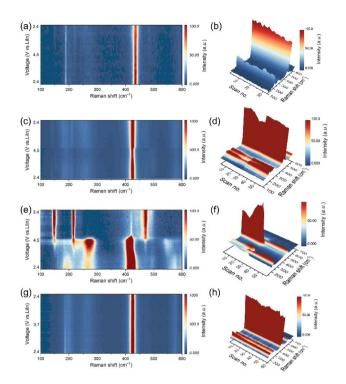
Fig. 2 The *in situ* Raman spectra of (a and b) LPSCI-VGCF|LPSCI|LiIn, (c and d) uncoated LNMO-LPSCI-VGCF|LPSCI|LiIn, (e and f) LTaP@LNMO-LPSCI-VGCF|LPSCI|LiIn, and (g and h) LCO-LPSCI-VGCF|LPSCI|LiIn cells from two-dimensional and three-dimensional views, respectively. The positions for Raman signal collection are the LPSCI-rich area far from the cathode active particle/LPSCI particle interface in the composite cathode.
