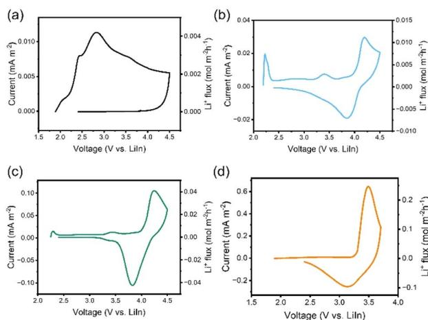
Fig. 1 The CV curves of (a) LPSCI-VGCF|LPSCI|LiIn, (b) uncoated LNMO-LPSCI-VGCF|LPSCI|LiIn, (c) LTA<sub>P</sub>@LNMO-LPSCI-VGCF|LPSCI|LiIn and (d) LCO-LPSCI-VGCF|LPSCI|LiIn cells, respectively. The battery used for measurement is newly assembled.
