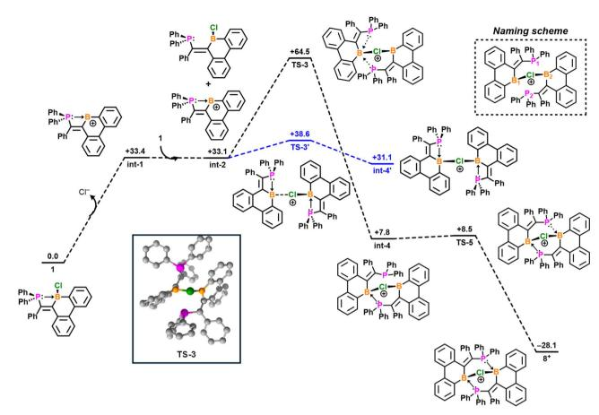
Fig. 7 Calculated relative free energies ( $\Delta G$ , kcal mol<sup>-1</sup>) for halide abstraction and subsequent ring expansion of compound **1** to form compound **8**<sup>+</sup> computed at the CPCM-B3LYP-D3-(BJ)/def2-TZVP level of theory. The dielectric constant ( $\epsilon$ ) was set to 5.42 to resemble fluorobenzene solvation.
