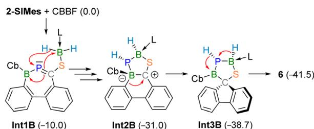
Scheme 5 Proposed mechanism for the formation of **6** from the reaction of **2-SIMes** with CBBF. Gibbs free energies in parentheses (kcal mol<sup>-1</sup>) are referenced to **2-SIMes** + CBBF and calculated at the B3LYP/D3(BJ)/def2SVP level of theory (solvent not included).
