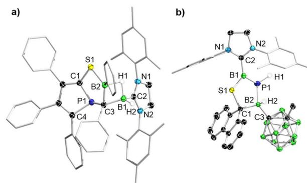
Fig. 3 Crystallography-derived solid-state structures of (a) **5** and (b) **6**. Atomic displacement ellipsoids set at 50% probability. Ellipsoids of ligand periphery and hydrogen atoms omitted for clarity except for B- and P-bound protons.
