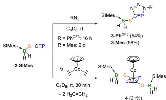
Scheme 2 Phosphaalkyne-like reactivity of **2-SIMes**. Ph<sup>CF<sub>3</sub></sup> = *p*-trifluoromethylphenyl. Mes = 2,4,6-trimethylphenyl.
