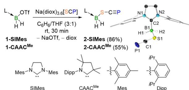
**Scheme 1** Synthesis of the carbene-stabilised phosphathioethynolato boranes **2-SIMes** and **2-CAAC<sup>Me</sup>**, and crystallography-derived solid-state structure of **2-SIMes**. Atomic displacement ellipsoids set at 50% probability. Ellipsoids of ligand periphery and hydrogen atoms omitted for clarity except for boron-bound hydrides. OTf = trifluoromethylsulfonate = triflate; diox = 1,4-dioxane.
