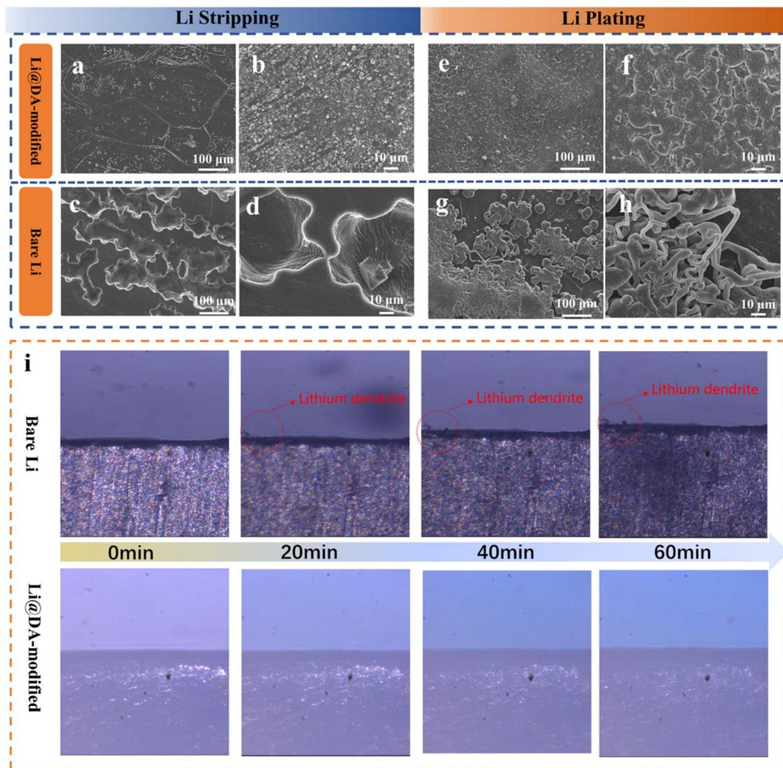
Fig. 3 SEM images of the deposition and stripping of bare Li and Li@DA symmetric cells after delithiation at  $0.25 \text{ mA cm}^{-2}$  for 6 hours: (a–d) Li@DA; (e–h) bare Li. (i) *In situ* optical microscopy measurements of bare Li and Li@DA at  $2 \text{ mA cm}^{-2}$ .
