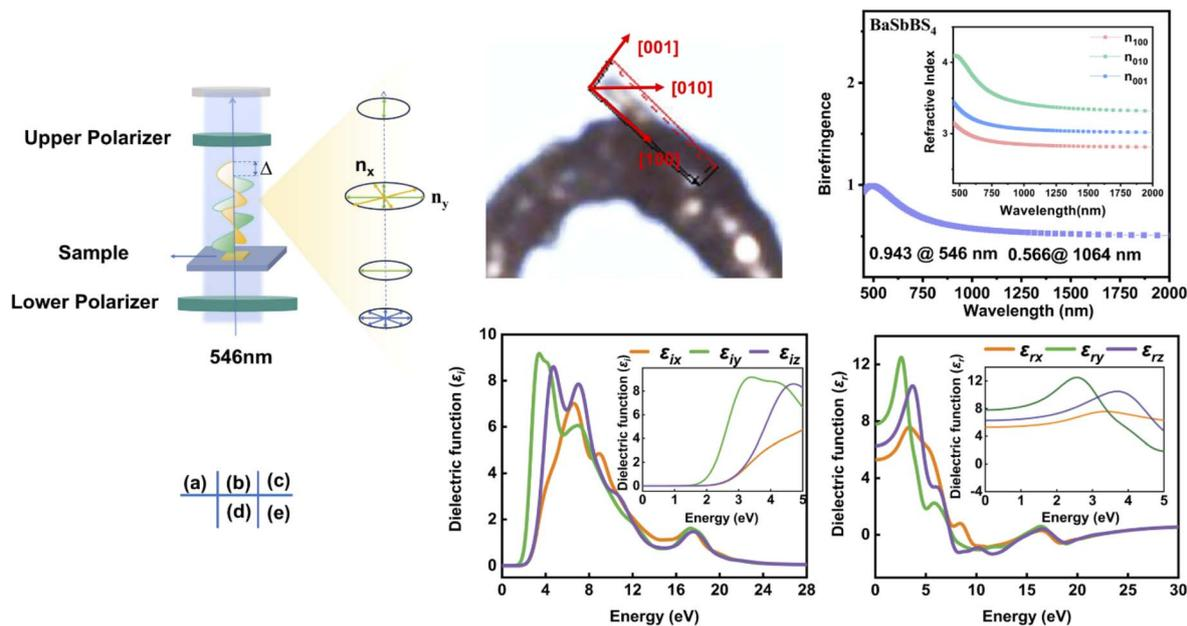
Fig. 6 (a) Schematic diagram for birefringence measurement. (b) Orientation of the BaSbBS<sub>4</sub> crystal determined by X-ray single-crystal diffraction. (c) Calculated refractive index and birefringence of BaSbBS<sub>4</sub>. (d) Imaginary parts of the dielectric function. (e) Real parts of the dielectric function.
