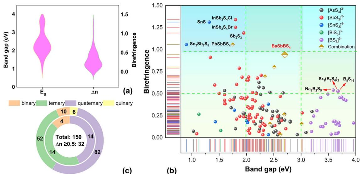
Fig. 4 (a) The violin map of band gap (eV) and  $\Delta n$ . (b) Birefringence-band gap map for all screened crystals (at 546 nm). (c) Distribution of stoichiometry of all screened crystals and highly birefringent ones among them.
