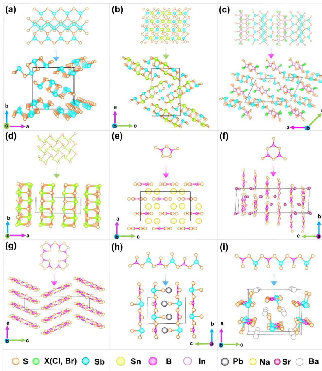
Fig. 5 Crystal structures of (a)  $\text{Sb}_2\text{S}_3$ , (b)  $\text{Sn}_2\text{Sb}_2\text{S}_5$ , (c)  $\text{InSb}_2\text{S}_4\text{X}$  ( $\text{X} = \text{Cl}, \text{Br}$ ), (d)  $\text{SnS}$ , (e)  $\text{Na}_2\text{B}_2\text{S}_5$ , (f)  $\text{Sr}_3(\text{B}_3\text{S}_6)_2$ , (g)  $\text{B}_8\text{S}_{16}$ , (h)  $\text{PbSbBS}_4$ , and (i)  $\text{BaSbBS}_4$ .
