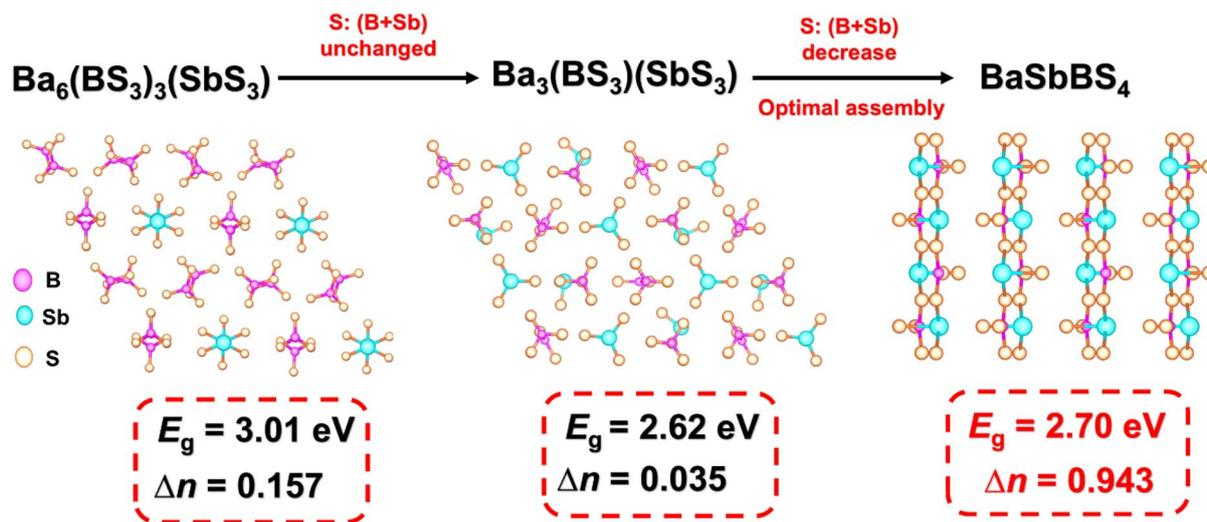
Fig. 7 Evolution from isolated  $[\text{BS}_3]^{3-}$  and  $[\text{SbS}_3]^{3-}$  motifs in  $\text{Ba}_6(\text{BS}_3)_3(\text{SbS}_3)$  and  $\text{Ba}_3(\text{BS}_3)(\text{SbS}_3)$  to the optimal assembled  $[\text{SbBS}_4]_{\infty}^{2-}$  chains in  $\text{BaSbBS}_4$ . The synergistic effect of FMs is activated.
