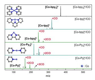
Fig. 6 Generality of the cluster model approach. Mass spectra for the reactions of CO with mass-selected [Co-bpy<sub>2</sub>]<sup>+</sup>, [Co-tpy]<sup>+</sup>, [Co-bpy]<sup>+</sup>, [Co-py]<sup>+</sup> at the reaction time of 30 ms, with optimized geometry of model clusters in their triplet ground state.
