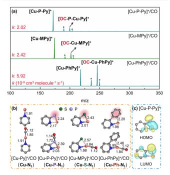
Fig. 4 Effects of doping/functional groups on the ortho carbon. (a) Mass spectra for the reactions of CO with mass-selected [CuL]<sup>+</sup> with rate constants (k in  $10^{-9}$  ( $\pm 30\%$ ) cm<sup>3</sup> molecule<sup>-1</sup> s<sup>-1</sup>) given in red. (b) Optimized geometry of model clusters and their CO-bound products in the ground state. (c) FMOs of [Cu-P-Py]<sup>+</sup>.
