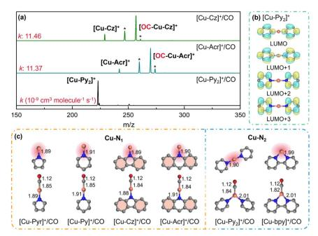
Fig. 3 Effects of N coordination configuration. (a) Mass spectra for the reactions of CO with mass-selected [CuL]<sup>+</sup> with rate constants (k in  $10^{-9}$  ( $\pm 30\%$ ) cm<sup>3</sup> molecule<sup>-1</sup> s<sup>-1</sup>) given in red. (b) LUMO + n (n = 0-3) of [Cu-Py<sub>2</sub>]<sup>+</sup>. (c) Optimized geometry of model clusters and their CO-bound products in the ground state.
