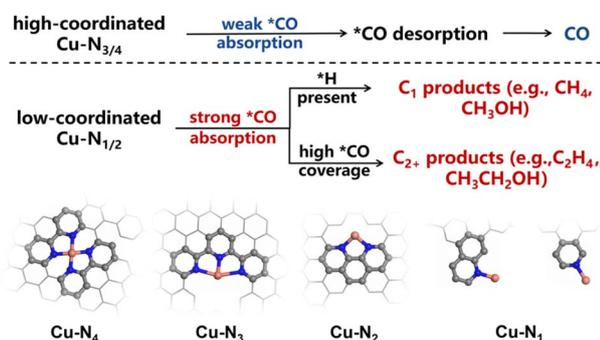
Scheme 1 Comparison of the catalytic mechanisms of \*CO adsorption at Cu-N<sub>x</sub> (x = 1–4) centers.
