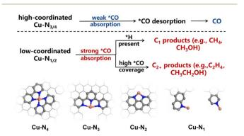
Scheme 1 Comparison of the catalytic mechanisms of \*CO adsorption at  ${\rm Cu-N_x}$  (x = 1–4) centers.
