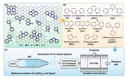
Fig. 1 Reaction apparatus and generation of Cu(i)-N-C model clusters. (a) Representative structures of the realistic Cu-N-C catalysts. (b) The ligands used in this study. (c) Schematic diagram of the mass spectrometry setup for the generation and reaction of model clusters.
