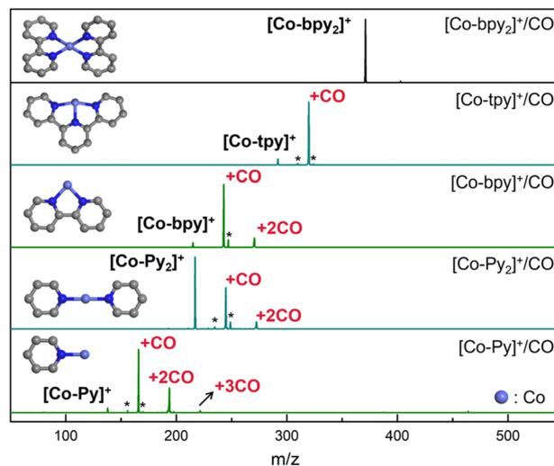
Fig. 6 Generality of the cluster model approach. Mass spectra for the reactions of CO with mass-selected [Co-bpy<sub>2</sub>]<sup>+</sup>, [Co-tpy]<sup>+</sup>, [Co-bpy]<sup>+</sup>, [Co-Py<sub>2</sub>]<sup>+</sup>, and [Co-Py]<sup>+</sup> at the reaction time of 30 ms, with optimized geometry of model clusters in their triplet ground state.
