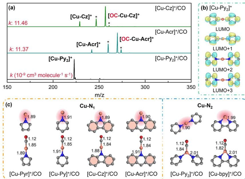
Fig. 3 Effects of N coordination configuration. (a) Mass spectra for the reactions of CO with mass-selected  $[\text{CuL}]^+$  with rate constants ( $k$  in  $10^{-9}$  ( $\pm 30\%$ )  $\text{cm}^3 \text{molecule}^{-1} \text{s}^{-1}$ ) given in red. (b) LUMO +  $n$  ( $n = 0-3$ ) of  $[\text{Cu-Py}_2]^+$ . (c) Optimized geometry of model clusters and their CO-bound products in the ground state.
