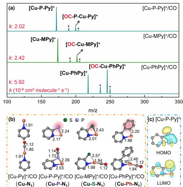
Fig. 4 Effects of doping/functional groups on the ortho carbon. (a) Mass spectra for the reactions of CO with mass-selected  $[\text{CuL}]^+$  with rate constants ( $k$  in  $10^{-9}$  ( $\pm 30\%$ )  $\text{cm}^3 \text{molecule}^{-1} \text{s}^{-1}$ ) given in red. (b) Optimized geometry of model clusters and their CO-bound products in the ground state. (c) FMOs of  $[\text{Cu-P-Py}]^+$ .
