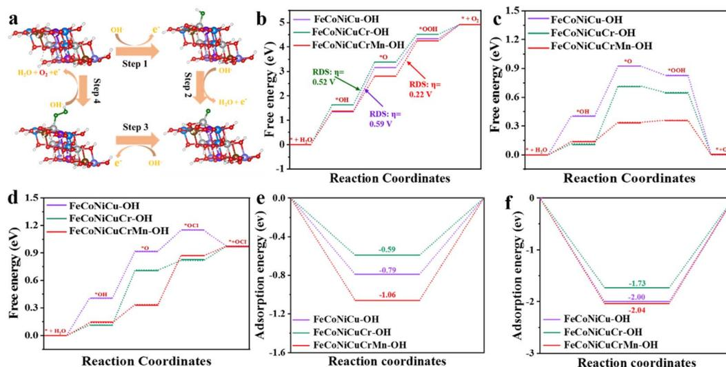
Fig. 6 (a) Proposed reaction mechanism of the OER on FeCoNiCuCrMn-OH. Reaction free energy diagrams for the (b) OER at  $U = 0$  V, (c) OER and (d) CER at  $U = 1.23$  V on different catalyst surfaces. Adsorption energy of (e)  $^*Cl$  and (f)  $^*OH$  on different catalyst surfaces.
