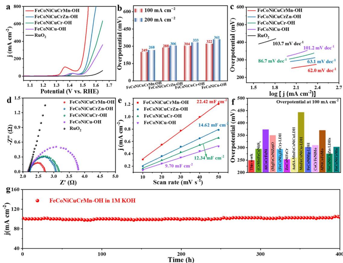
Fig. 4 (a) OER LSV curves, (b) overpotential comparison, (c) Tafel slope values, (d) Nyquist plots, (e) double-layer capacitance ( $C_{dl}$ ) measurements, (f) comparison of overpotentials (at  $100 \text{ mA cm}^{-2}$ ) of FeCoNiCuCrMn-OH with other electrocatalysts, and (g) the long-term stability test of FeCoNiCuCrMn-OH at  $100 \text{ mA cm}^{-2}$  in 1.0 M KOH.
