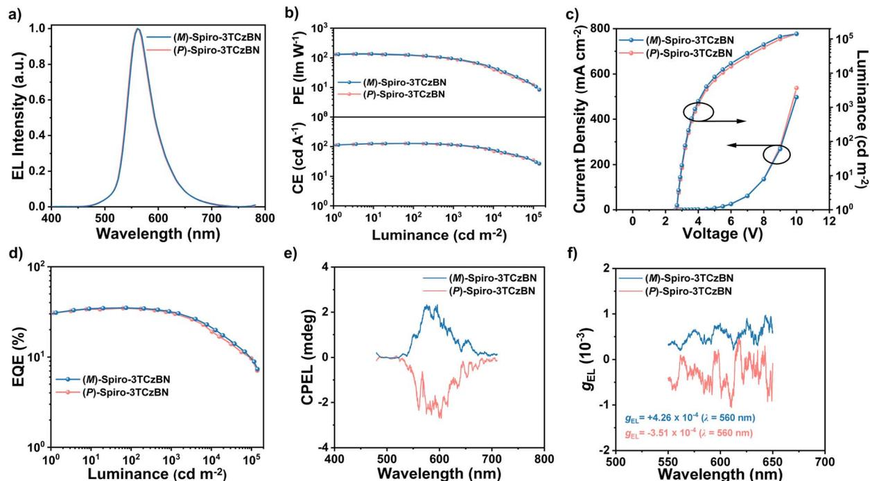
Fig. 5 EL characteristics of the devices with a sensitizer based on (*P/M*)-Spiro-3TCzBN. (a) EL spectra. (b)  $J$ - $V$ - $L$  curves. (c) EQE- $L$  curves. (d) CE- $L$ , PE- $L$  curves. (e) CPEL curves. (f)  $g_{EL}$  curves.
