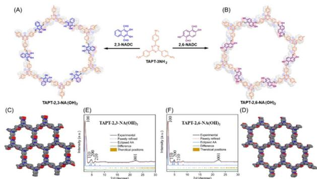
Fig. 15 (A and B) Structures of TAPT-2,3-NA(OH)<sub>2</sub> and TAPT-2,6-NA(OH)<sub>2</sub> COFs. Top-view crystal structures of (C) TAPT-2,3-NA(OH)<sub>2</sub> and (D) TAPT-2,6-NA(OH)<sub>2</sub> COFs. Experimental and simulated PXRD patterns of (E) TAPT-2,3-NA(OH)<sub>2</sub> and (F) TAPT-2,6-NA(OH)<sub>2</sub> COFs. Reproduced from ref. 103 with permission from [MDPI], Copyright [2022].
