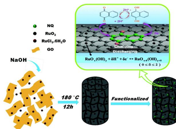
Fig. 13 Schematic presentation of the synthesis of the NQ-RuO<sub>2</sub>/SGH composite electrode material. Reproduced from ref. 96 with permission of RSC.
