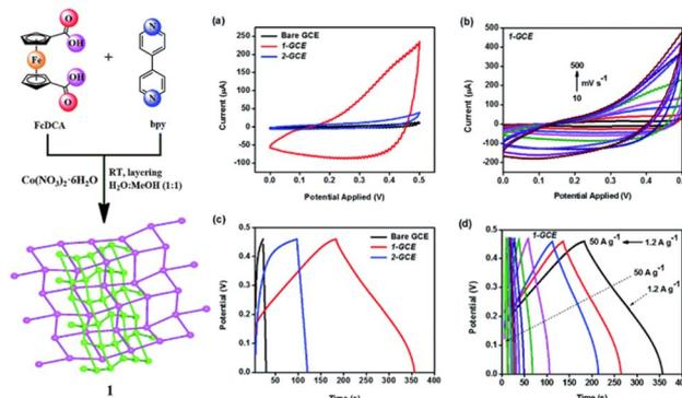
Fig. 54 Structure of Fc-MOF-1 and (a) CV curves of base GCE, 1-GCE and 2-GCE at  $100 \text{ mV s}^{-1}$ ; (b) CV curves of 1-GCE at different scan rates ( $10$  to  $500 \text{ mV s}^{-1}$ ); (c) GCD profiles of base GCE, 1-GCE and 2-GCE at  $1.2 \text{ A g}^{-1}$ ; and (d) GCD profiles of 1-GCE at different current densities ranging from  $1.2$  to  $50 \text{ A g}^{-1}$  in  $1 \text{ M KOH}$  electrolyte solution. Reproduced from ref. 268 with permission from RSC.
