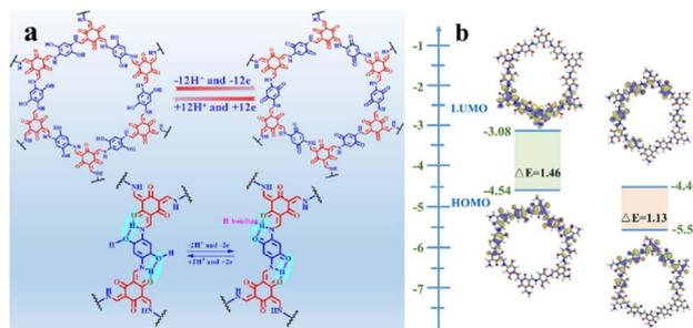
Fig. 12 (a) Plausible reversible faradaic redox-activity of (TpPa-(OH)<sub>2</sub>) and (b) corresponding HOMO and LUMO energy levels of (TpPa-(OH)<sub>2</sub>) in the charge–discharge process. Reproduced from ref. 89b with permission from [Elsevier], Copyright [2024].
