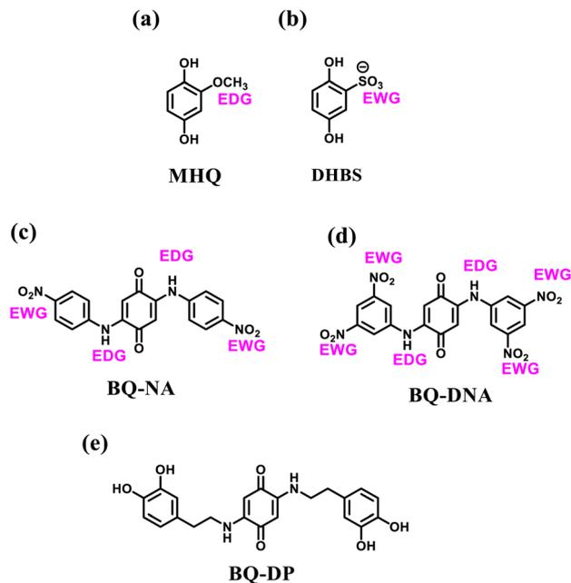
Fig. 7 Functionalized hydroquinone and quinone: (a) MHQ, (b) DHBS, (c) BQ-NA, (d) BQ-DNA and (e) BQ-DP for supercapacitor applications.
