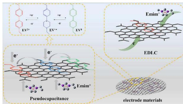
Fig. 60 Charge-storage mechanisms of EV<sub>20</sub>-RGO on the negative electrodes. Reproduced from ref. 292 with permission from [Elsevier], Copyright [2023].
