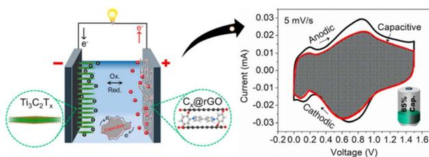
Fig. 62 ASC device architecture based on quinone-functionalized viologen ( $\text{C}_x\text{@rGO}$ ) as the positive electrode and  $\text{Ti}_3\text{C}_2\text{T}_x$  MXene as the negative electrode and the energy storage mechanism. Reproduced from ref. 294 with permission from [Elsevier], Copyright [2020].
