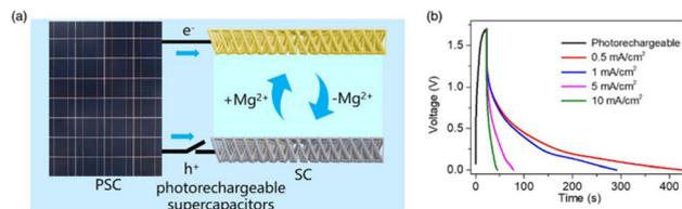
Fig. 42 (a) Working principle of photo-rechargeable supercapacitors and (b) GCD profiles of photo-rechargeable supercapacitors. Reproduced from ref. 212 with permission from [John Wiley and Sons], Copyright [2023].
