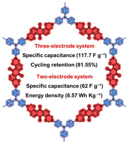
Fig. 24 Structure of An-TPT porous organic polymer (POP) and its properties in three-electrode and two-electrode SC systems. Reproduced from ref. 140 with permission from [Elsevier], Copyright [2024].
