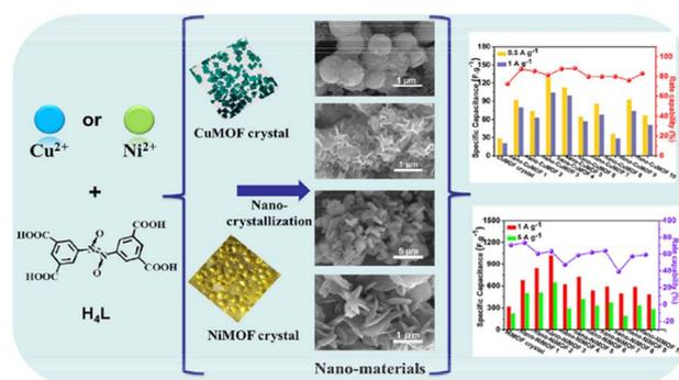
Fig. 45 Molecular structure of 3,5-dicarboxyl-(3',5'-dicarboxylazophenyl)benzene acid H<sub>4</sub>L ligand, SEM images of MOF nano-materials and specific capacitance of the CuMOF crystal and NiMOF crystal. Reproduced from ref. 232 with permission from [Elsevier], Copyright [2020].
