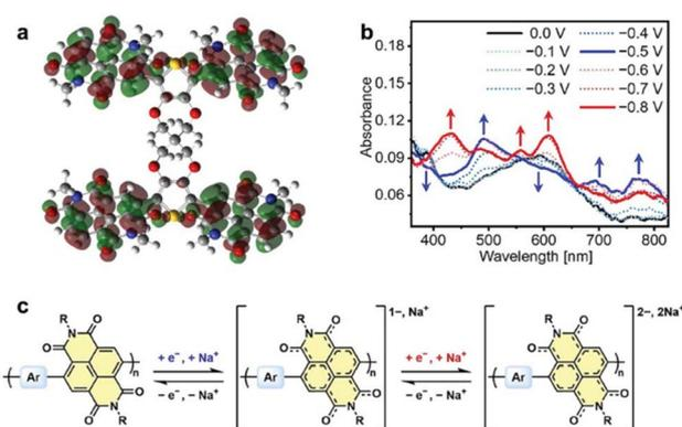
Fig. 37 Spiro-NDI-N-based pseudocapacitive energy storage mechanism. (a) LUMO of spiro-NDI-N; (b) spectroelectrochemical measurements of spiro-NDI-N film in aqueous  $2$  M NaCl electrolyte at an applied potential in the range of  $0.0$  V to  $-0.8$  V; and (c) proposed pseudocapacitive charge storage mechanism of polymers based on NDIs. Reproduced from ref. 195 with permission from [John Wiley and Sons], Copyright [2024].
