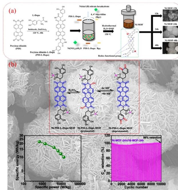
Fig. 33 (a) Schematic illustration of the preparation of Ni-MOF, (b) redox-mechanism of Ni-MOF and Ragone plot and cycling stability. Reproduced from ref. 178 with permission from [Elsevier], Copyright [2023].
