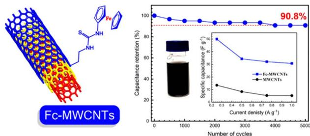
Fig. 47 Structural unit of ferrocene-functionalized MWCNTs and capacitance retention after 5000 GCD cycles (inset shows the variation of  $C_{\text{sp}}$  with current density). Reproduced from ref. 242 with permission from [Elsevier], Copyright [2020].
