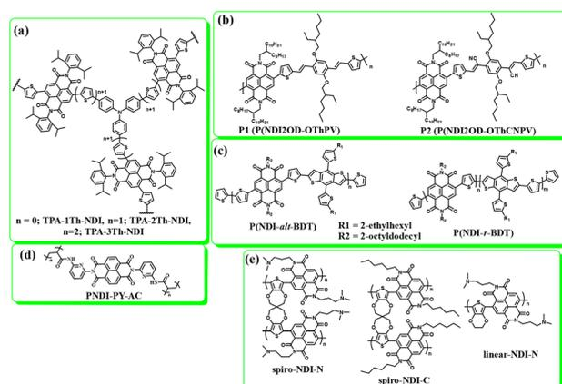
Fig. 36 Molecular structure of various polymers (a) TPA-1Th-NDI, TPA-2Th-NDI, TPA-3Th-NDI, (b) P1 (P(NDI2OD-OTHPV)), P2 (P(NDI2OD-OTHCNPV)), (c) P(NDI-*alt*-BDT), P(NDI-*r*-BDT), (d) PNDI-Py-AC and (e) spiro-NDI-N, spiro-NDI-C, linear-NDI-N based on naphthalene diimide (NDI).
