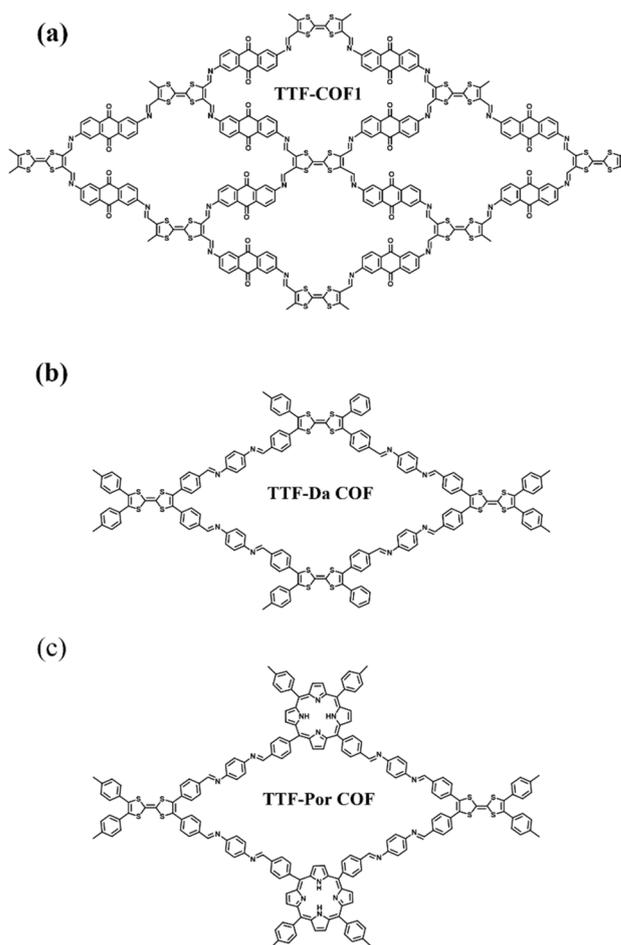
Fig. 56 (a–c) Different structures of TTF-based COFs.
