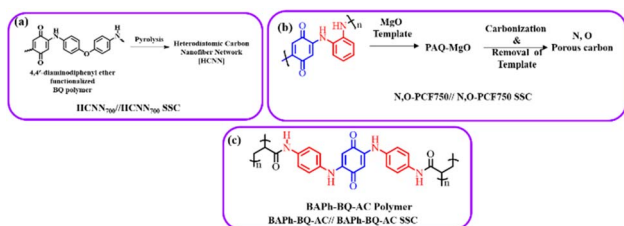
Fig. 9 Benzoquinone (BQ)-based polymer structures and materials: (a) HCNN 700 , (b) N,O-PCF 750 and (c) BAPh-BQ-AC.
