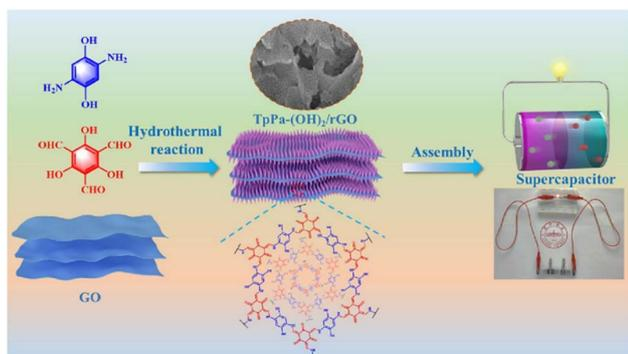
Fig. 11 Schematic of the preparation of the (TpPa-(OH)<sub>2</sub>)/rGO material, its assembly in an SC device and three SCs applied to light an LED lamp. Reproduced from ref. 89b with permission from [Elsevier], Copyright [2024].
