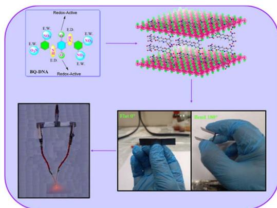
Fig. 8 Schematic presentation of the molecular structure of BQ-DNA and the BQ-DNA/rGO composite, flexible device and illumination of LED light at  $1.8 \text{ V}$ . Reproduced from ref. 77 with permission from [the American Chemical Society], Copyright [2024].
