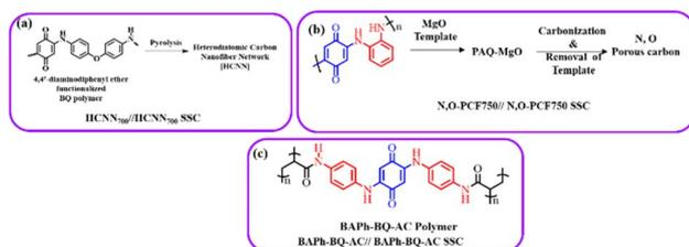
Fig. 9 Benzoquinone (BQ)-based polymer structures and materials: (a) HCNN<sub>700</sub>, (b) N,O-PCF<sub>750</sub> and (c) BAPh-BQ-AC.
