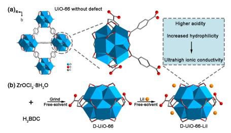
Scheme 1 (a) Illustration of UiO-66 without defects. (b) Schematic illustration of the preparation of D-UiO-66-Lil.
