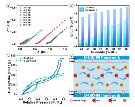
Fig. 2 (a) Nyquist plots of D-UiO-66-Lil at 30 °C and different humidities varying from 40% to 98% RH. (b) Ionic conductivities of D-UiO-66 and D-UiO-66-Lil at 30 °C and different humidities varying from 40% to 98% RH. (c) H<sub>2</sub>O vapor adsorption–desorption isotherms of D-UiO-66 and D-UiO-66-Lil at 298 K. (d) Schematic illustration of ionic transport in D-UiO-66-Lil under humidity conditions.
