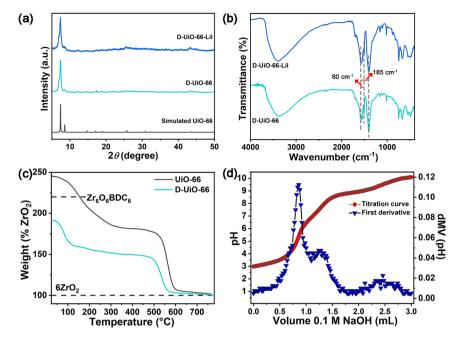
Fig. 1 (a) PXRD patterns of simulated UiO-66, D-UiO-66, and D-UiO-66-Lil. (b) FT-IR spectra of D-UiO-66 and D-UiO-66-Lil. (c) TGA curves of UiO-66 and D-UiO-66. The end weight of ZrO<sub>2</sub> is normalized to 100%. (d) Acid-base titration curve and first derivative curve for D-UiO-66.
