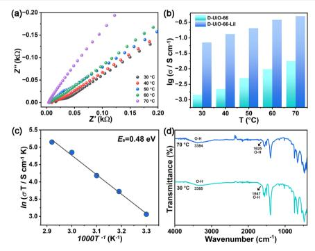
Fig. 3 (a) Nyquist plots of D-UiO-66-Lil at 98% RH and different temperatures varying from 30 to 70 °C. (b) Ionic conductivities of D-UiO-66 and D-UiO-66-Lil at 98% RH and different temperatures varying from 30 to 70 °C. (c) Arrhenius plot of D-UiO-66-Lil at 98% RH and in the temperature range of 30-70 °C. (d) Temperature-dependent FT-IR spectra of D-UiO-66-Lil.
