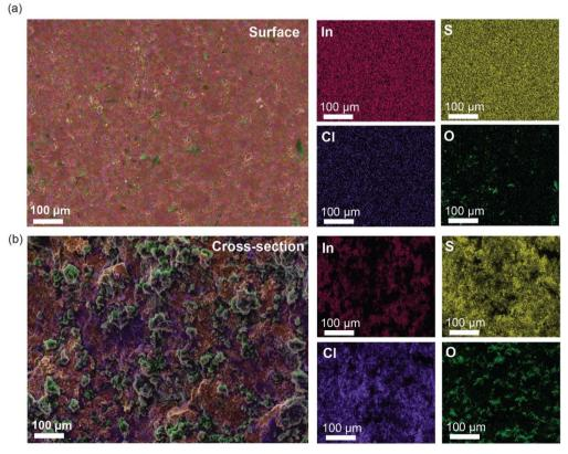
Fig. 7 SEM image and EDS elemental mapping of In, S, Cl, and O for the (a) surface (b) cross-section of Li<sub>3.6</sub>In<sub>7</sub>S<sub>11.8</sub>Cl pellet dried at 150 °C.
