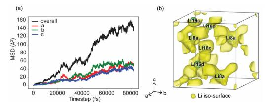
Fig. 4 (a) Mean square displacements of  $\text{Li}^+$  in  $\text{Li}_{3.6}\text{In}_7\text{S}_{11.8}\text{Cl}$  generated from AIMD simulations at 900 K. (b)  $\text{Li}^+$  (yellow) probability density distribution in  $\text{Li}_{3.6}\text{In}_7\text{S}_{11.8}\text{Cl}$  in a  $1\times1\times1$  supercell based on the AIMD simulations at 900 K.
