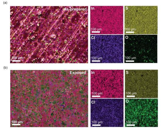
Fig. 6 SEM images and EDS elemental mapping of In, S, Cl, and O for (a) as-prepared and (b) moisture-exposed Li<sub>3.6</sub>In<sub>7</sub>S<sub>11.8</sub>Cl.
