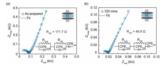
Nyquist plots and equivalent circuit fitting of (a) as-prepared Li<sub>3.6</sub>In<sub>7</sub>S<sub>11.8</sub>Cl and (b) moisture-exposed Li<sub>3.6</sub>In<sub>7</sub>S<sub>11.8</sub>Cl.
