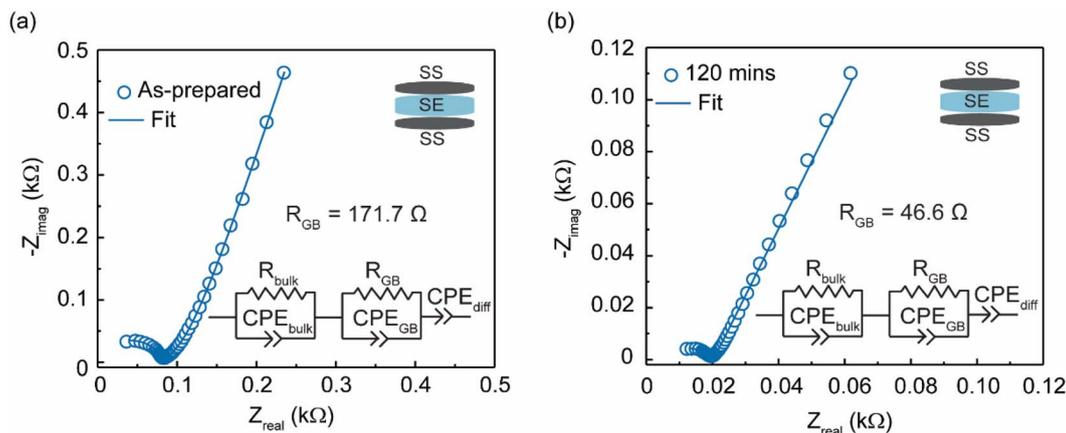
Fig. 8 Nyquist plots and equivalent circuit fitting of (a) as-prepared  $\text{Li}_{3.6}\text{In}_7\text{S}_{11.8}\text{Cl}$  and (b) moisture-exposed  $\text{Li}_{3.6}\text{In}_7\text{S}_{11.8}\text{Cl}$ .
