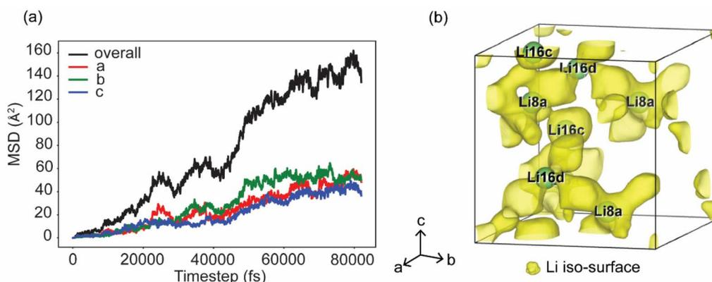
Fig. 4 (a) Mean square displacements of  $\text{Li}^+$  in  $\text{Li}_{3.6}\text{In}_7\text{S}_{11.8}\text{Cl}$  generated from AIMD simulations at 900 K. (b)  $\text{Li}^+$  (yellow) probability density distribution in  $\text{Li}_{3.6}\text{In}_7\text{S}_{11.8}\text{Cl}$  in a  $1 \times 1 \times 1$  supercell based on the AIMD simulations at 900 K.
