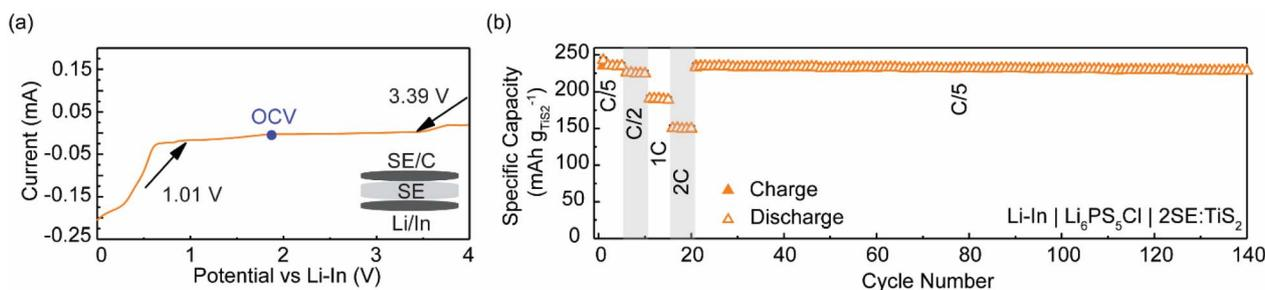
Fig. 9 (a) Linear sweep voltammetry (current–voltage) plot of  $\text{Li}_{3.6}\text{In}_7\text{S}_{11.8}\text{Cl}$  (b) the rate performance and long-term cycling stability of a  $\text{Li-In|Li}_6\text{PS}_5\text{Cl|}2\text{SE:TiS}_2$  cell (SE =  $\text{Li}_{3.6}\text{In}_7\text{S}_{11.8}\text{Cl}$ ).  $C = 239 \text{ mA h g}^{-1}$ .
