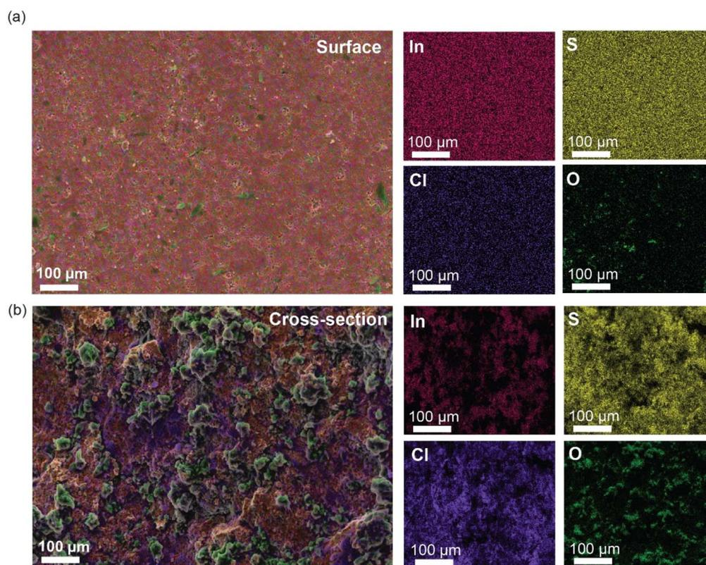
Fig. 7 SEM image and EDS elemental mapping of In, S, Cl, and O for the (a) surface (b) cross-section of  $\text{Li}_{3.6}\text{In}_7\text{S}_{11.8}\text{Cl}$  pellet dried at  $150 \text{ }^\circ\text{C}$ .
