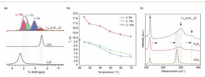
Fig. 2 (a)  $^6$ Li NMR spectra with resonance assignment.  $^6$ Li spectra of LiCl and Li<sub>2</sub>S are shown as references. (b)  $^7$ Li  $T_1$  NMR relaxation times of Li<sub>3.6</sub>In<sub>7</sub>S<sub>11.8</sub>Cl as a function of temperature, revealing faster ion dynamics of Li<sub>8a</sub> and Li<sub>16c</sub>, compared with Li<sub>16d</sub>. (c) Raman spectra of as-prepared  $Li_{3.6}In_7S_{11.8}Cl$ ,  $In_2S_3$ , and  $InCl_3$ .
