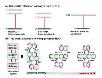
Fig. 1 (a) Illustration of relaxation pathways of a D-A-type  $\pi$ -conjugated system from the excited state  $(S_1)$  to the ground state  $(S_0)$ . (b) Scheme of geometrical twisting-governed HLCT character of APAH-
