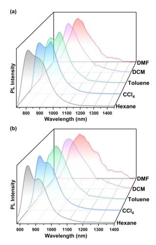
Fig. 5 Photoluminescence profiles of (a) APAH-b and (b) APAH-c in solvents (1  $\times$  10<sup>-5</sup> M) with varying polarities.
