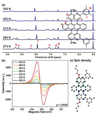
Fig. 4 (a) Variable-temperature  $^1H$  NMR spectra (aromatic region) of APAH-c recorded in  $C_2D_2Cl_4$  (the chemical shift of the solvent molecule is at 6.00 ppm). (b) Variable-temperature ESR spectra of APAH-c in solid state. (c) The Mulliken spin density distribution of APAH-c (isovalue = 0.008).
