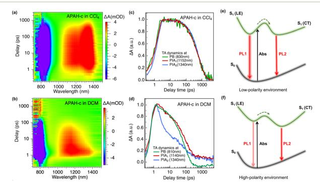
Fig. 6 Pseudo-color representation of fs-TA spectra of APAH-c recorded in  $CCl_4$  (a) and DCM (b) following photoexcitation at 400 nm. TA decay dynamics of ground-state photo-bleaching (PB) at 830 nm and photo-induced absorptions (PIAs) for APAH-c in  $CCl_4$  (c) and DCM (d). Schematic relaxation pathways in low-polarity (e) and high-polarity (f) solvents after excitation.
