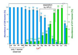
Fig. 3 Compositions of the final reaction mixtures after synthesis (pH 6-7 and 60 °C) of the Ln(III)-H<sub>4</sub>pyta complexes determined by analytical HPLC. The 22 isomers are in blue and the 21 isomers are in green. The error bars and the average abundances are based on three independent preparations
