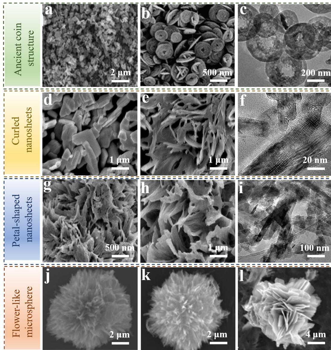
Fig. 4 (a–c)  $\text{VO}_2$  nanosheets with an ancient coin structure.<sup>64</sup> Copyright 2020, Wiley-VCH GmbH. (d–f) Curled  $\text{VO}_2$  nanosheets.<sup>65</sup> Copyright 2023, Elsevier. (g–i) Petal-shaped folded  $\text{VO}_2$  nanosheets.<sup>66</sup> Copyright 2022, Elsevier. (j–l) Hierarchical flower-shaped  $\text{VO}_2$  nanosheets.<sup>67</sup> Copyright 2023, Wiley-VCH.
