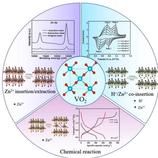
Fig. 5 Schematic diagram of three energy storage mechanisms of a VO<sub>2</sub>-based cathode for AZIBs.<sup>69</sup> Copyright 2019, American Chemical Society.<sup>72</sup> Copyright 2021, Wiley-VCH.<sup>74</sup> Copyright 2021, Elsevier.
