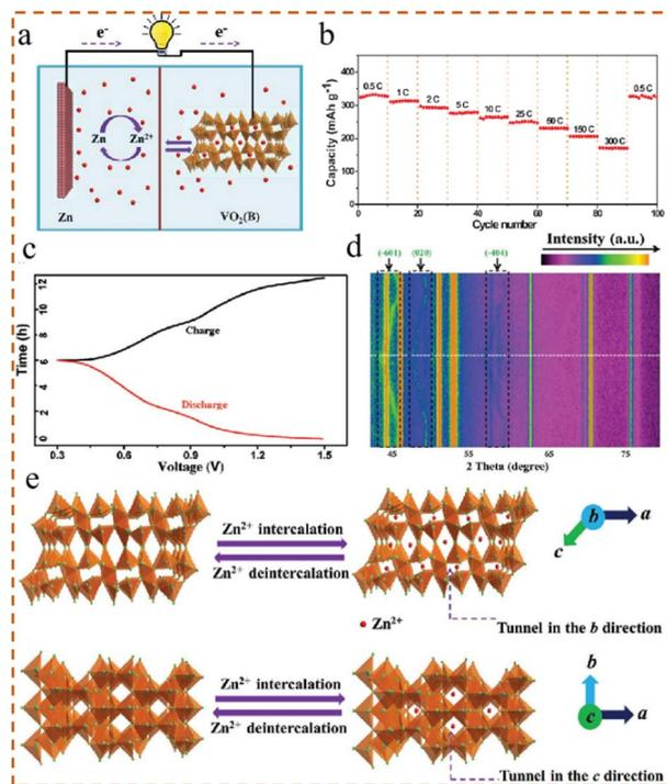
Fig. 6 (a) Crystal structure of VO<sub>2</sub> and battery schematic. (b) Rate performance of VO<sub>2</sub>. (c) Charge–discharge curve of VO<sub>2</sub> at 0.5C. (d) *In situ* XRD pattern of VO<sub>2</sub>. (e) Schematic diagram of Zn<sup>2+</sup> embedded in different crystal planes of VO<sub>2</sub>.<sup>70</sup> Copyright 2018, Wiley-VCH.
