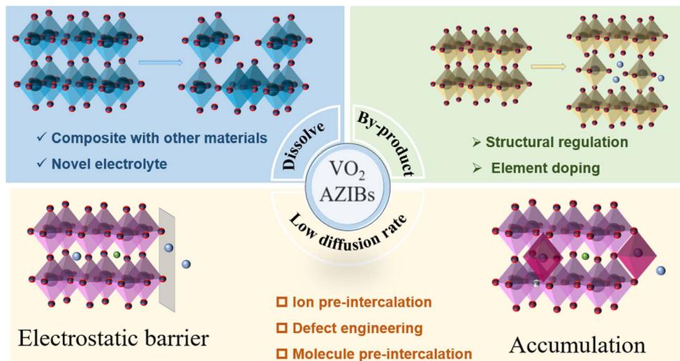
Fig. 9 The main problems and strategies of VO<sub>2</sub>-based cathode materials for AZIBs.
