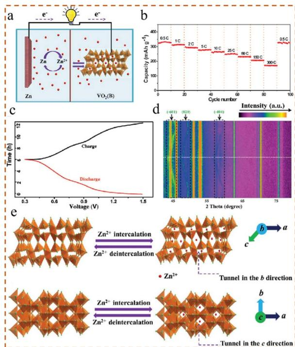
Fig. 6 (a) Crystal structure of  $\text{VO}_2$  and battery schematic. (b) Rate performance of  $\text{VO}_2$ . (c) Charge–discharge curve of  $\text{VO}_2$  at 0.5C. (d) *In situ* XRD pattern of  $\text{VO}_2$ . (e) Schematic diagram of  $\text{Zn}^{2+}$  embedded in different crystal planes of  $\text{VO}_2$ .<sup>70</sup> Copyright 2018, Wiley-VCH.
