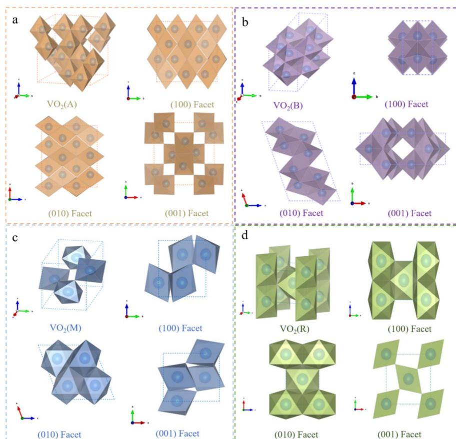
Fig. 2 The lattice structures of VO<sub>2</sub>: (a) VO<sub>2</sub>(A), (b) VO<sub>2</sub>(B), (c) VO<sub>2</sub>(M), and (d) VO<sub>2</sub>(R), each viewed from different facets.
