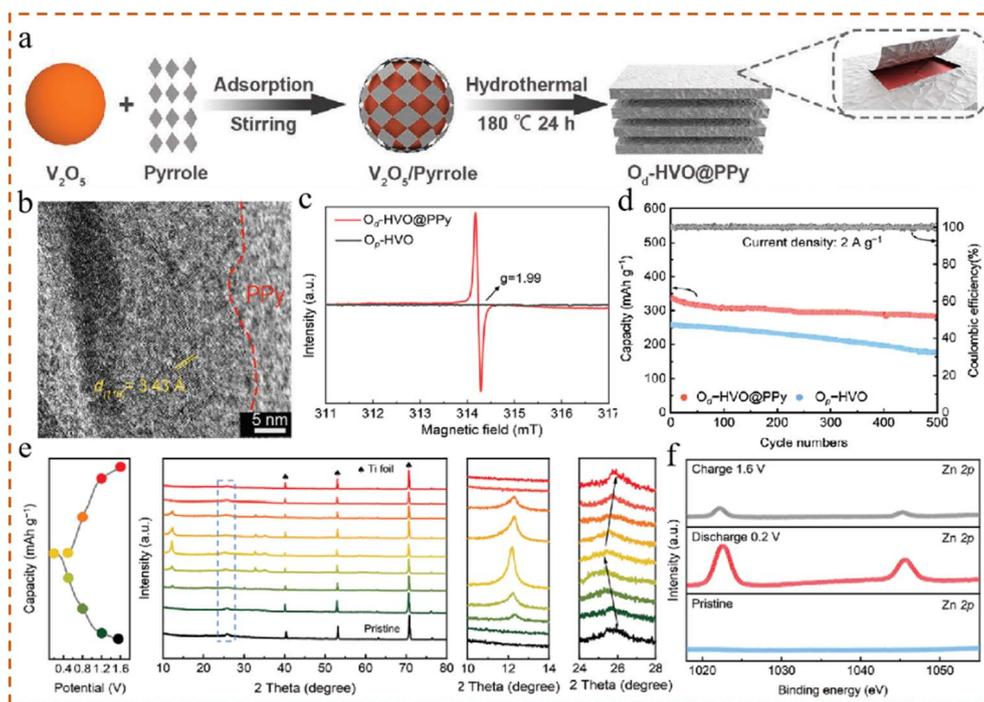
Fig. 7 (a) Schematic diagram of the synthesis of  $O_d$ -HVO@PPy, (b) HRTEM of  $O_d$ -HVO@PPy, (c) electron paramagnetic resonance of  $O_d$ -HVO@PPy, (d) long-cycle curves of  $O_d$ -HVO@PPy and  $O_p$ -HVO electrodes at  $2 \text{ A g}^{-1}$ , (e) *ex situ* XRD of the  $O_d$ -HVO@PPy electrode in selected states of the 2<sup>nd</sup> cycle, and (f) XPS spectra of Zn 2p in the 2<sup>nd</sup> cycle.<sup>72</sup> Copyright 2021, Wiley-VCH.
