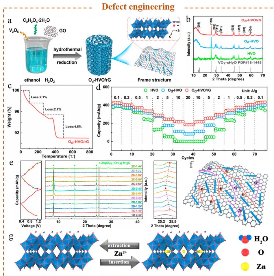
Fig. 14 (a) Schematic diagram of the synthesis of  $O_d$ -HVO/rG materials, (b) XRD patterns of all samples, (c) TGA curve of  $O_d$ -HVO/rG, (d) rate performance of HVO,  $O_d$ -HVO and  $O_d$ -HVO/rG, (e) *ex situ* XRD of  $O_d$ -HVO/rG, and (f and g) schematic diagram of the energy storage mechanism of  $O_d$ -HVO/rG.<sup>108</sup> Copyright 2021, American Chemical Society.
