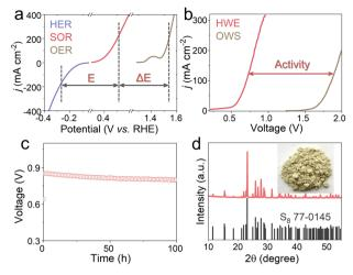
Fig. 5 (a) Voltage difference between the HER and SOR/OER. (b) Polarization curves of HWE and OWS systems for Fe-Ni $_{0.85}$ Se. (c) Durability test of the HWE process. (d) XRD pattern of the S product. Inset: Digital image of S.
