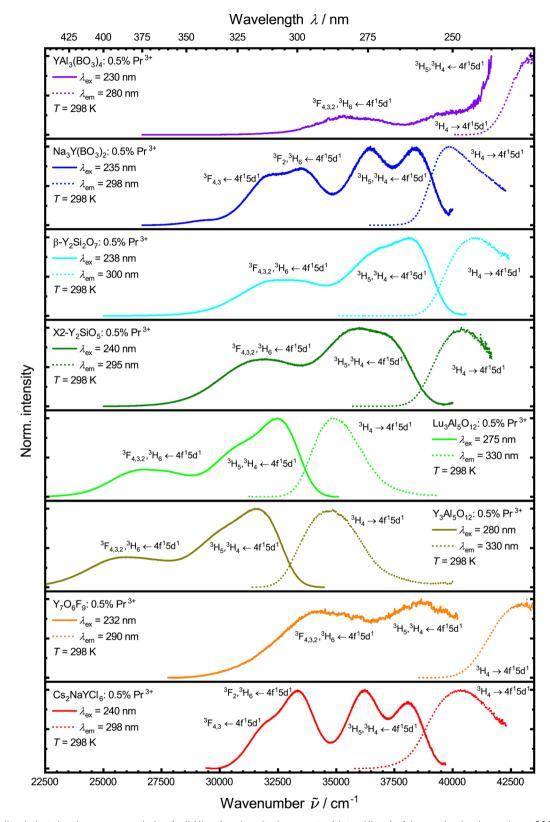
Fig. 5 Normalized photoluminescence emission (solid lines) and excitation spectra (dotted lines) of the synthesized samples at 298 K in UV range showing emission and excitation of  $4f^15d^1$  states. Spectra were measured against wavelengths and converted to wavenumbers using a Jacobian transformation.<sup>99</sup>
