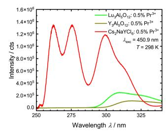
Fig. 10 Comparison of the intensities of the UC luminescence of Pr<sup>3+</sup> in LuAG, YAG and Cs<sub>2</sub>NaYCl<sub>6</sub> measured under the same conditions (under air at 298 K) and with the same measurement parameters (1 nm emission bandwidth, 0.1 nm step size, 0.3 s dwell time).
