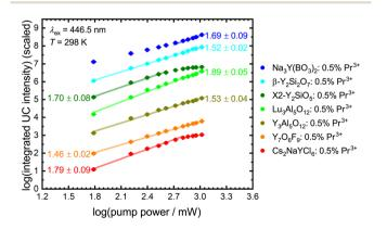
Fig. 8 Double logarithmic plot of integrated intensity of the upconverted  $4f^15d^1$ -based emission of  $Pr^{3+}$  against blue laser ( $\lambda_{\rm ex}=446.5$  nm) pump power at 298 K with linear regression. UC intensity is scaled to allow a better comparison. Slopes are given in the diagram.
