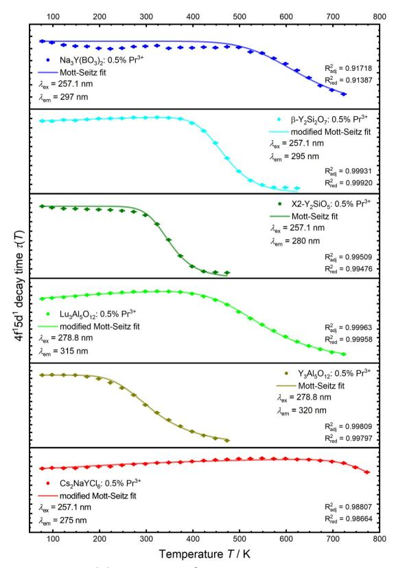
Fig. 6 Luminescence decay times of  $4f^15d^1$  configuration states of  $Pr^{3+}$  in the synthesized host compounds as a function of temperature with a fit to a Mott-Seitz law (eqn (1) or (3)). Decay times were derived from the exponential fit using eqn (S1).†
