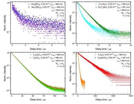
Fig. 4 Photoluminescence decay curves of the synthesized samples of the  $^3P_0$  level under 450.9 nm excitation ( $^3P_2 \leftarrow ^3H_4$ ) at 77 K monitoring the  $^3P_0 \rightarrow ^3H_4$ -based emission around 488 nm. Due to strongly differing decay times, decay curves are shown for different delay times. Values of the measured decay times are given in Table 1.
